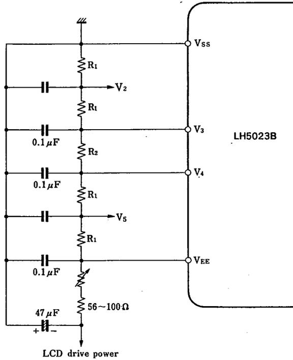
Note: Be sure to apply  $56\Omega$  to  $100\Omega$  of a resistor to the LCD drive power supply.
