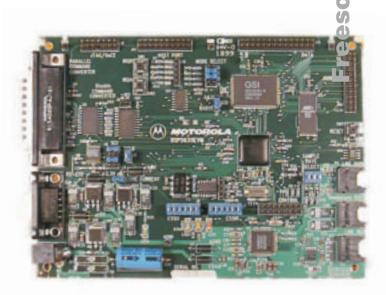
The DSP56311EVM is shipped with all the jumper blocks in the default configuration. The photo on the left shows the default configuration for your reference.
