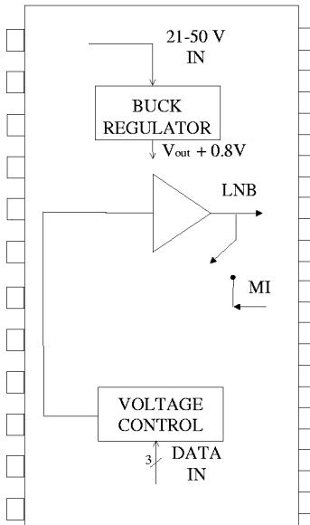
*LNB Supply and Control Voltage Regulator*
