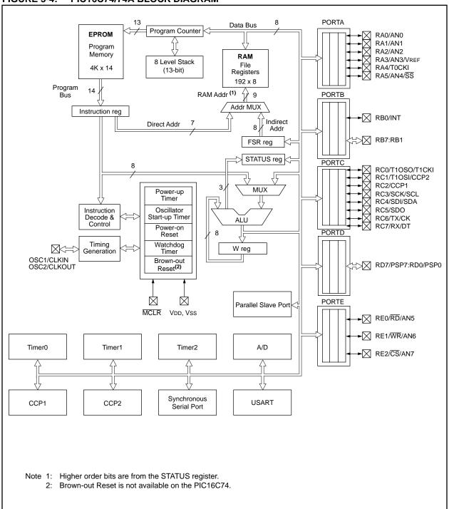
FIGURE 3-4: PIC16C74/74A BLOCK DIAGRAM
