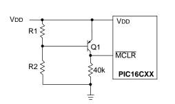
Note 1: This brown-out circuit is less expensive, albeit less accurate. Transistor Q1 turns off when VDD is below a certain level such that:
