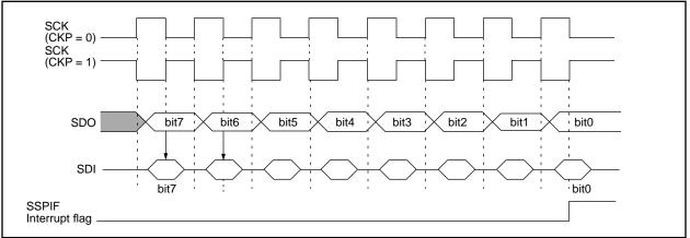
FIGURE 11-5: SPI MODE TIMING (MASTER MODE OR SLAVE MODE W/O SS CONTROL)
