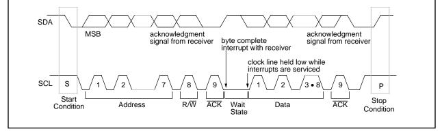
Figure 11-12 and Figure 11-13 show Master-transmitter and Master-receiver data transfer sequences.
