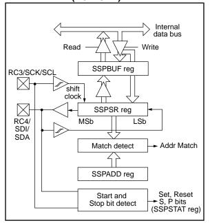
The SSP module has five registers for  $l^2C$  operation. These are the:
