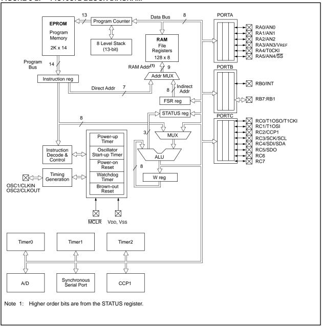
FIGURE 3-2: PIC16C72 BLOCK DIAGRAM
