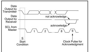
If the master is receiving the data (master-receiver), it generates an acknowledge signal for each received byte of data, except for the last byte. To signal the end of data to the slave-transmitter, the master does not generate an acknowledge (not acknowledge). The slave then releases the SDA line so the master can generate the STOP condition. The master can also generate the STOP condition during the acknowledge pulse for valid termination of data transfer.
