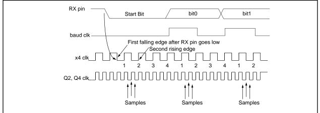
FIGURE 12-5: RX PIN SAMPLING SCHEME (BRGH = 1)
