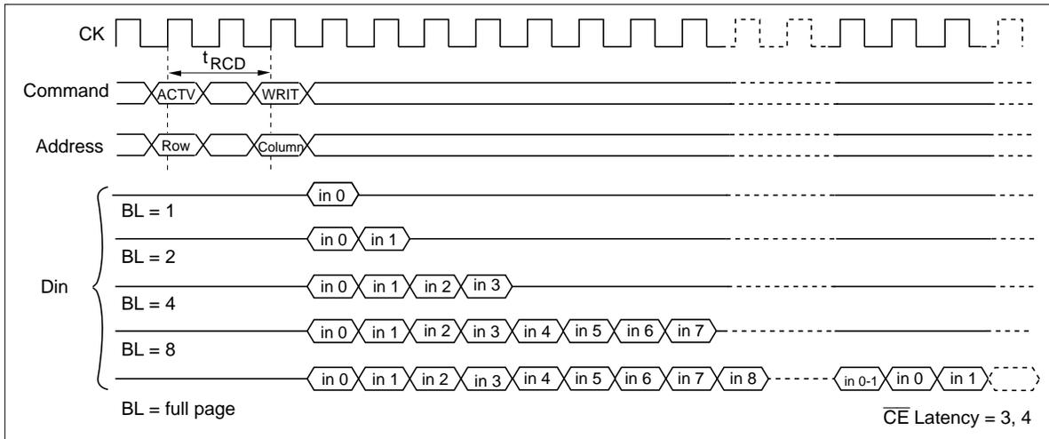
**2. Single write:** A single write operation is enabled by setting OPCODE (A9, A8) to (1, 0). In a single write operation, data is only written to the column address and the bank select address (BA) specified by the write command set cycle without regard to the burst length setting. (The latency of data input is 1 clock).
