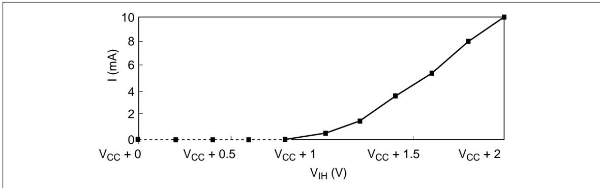
**$I_{OL}/I_{OH}$  Characteristics (Component characteristics)****Output Low Current ( $I_{OL}$ )**
