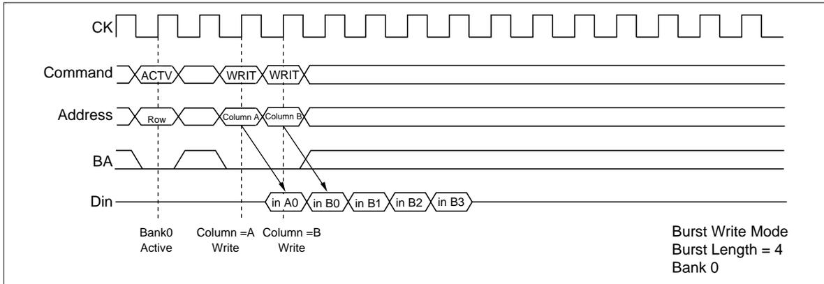
**2. Same bank, different ROW address:** When the ROW address changes, consecutive write commands cannot be executed; it is necessary to separate the two write commands with a precharge command and a bank-active command.
