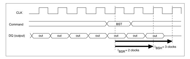
**Burst stop command at burst write:** The burst stop command (BST command) is used to stop data input during a full-page burst write. No data is written in the same clock as the BST command, and in subsequent clocks. In addition, the BST command is only valid during full-page burst mode, and is illegal with burst lengths of 1, 2, 4 and 8. And an interval of  $t_{DPL}$  is required between last data-in and the next precharge command.
