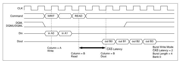
**2. Same bank, different ROW address:** When the ROW address changes, consecutive read commands cannot be executed; it is necessary to separate the two commands with a precharge command and a bank-active command.
