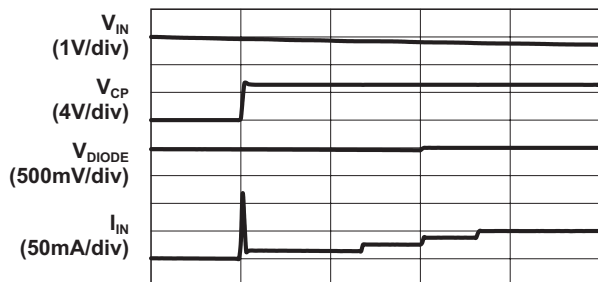
Load Switch to Charge Pump (1.5X Mode; 4x19mA Load)
