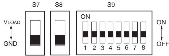
Figure 3-15. Port 11 Mask Option Setting (At Shipment)
