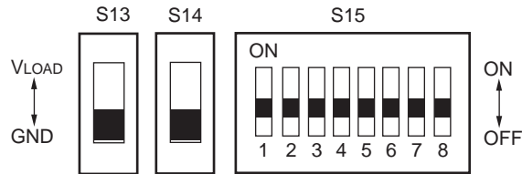
Figure 3-16. Port 10 Mask Option Setting (At Shipment)
