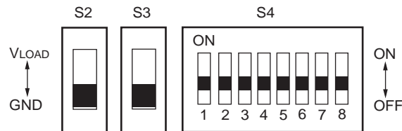
Figure 3-14. Port 12 Mask Option Setting (At Shipment)
