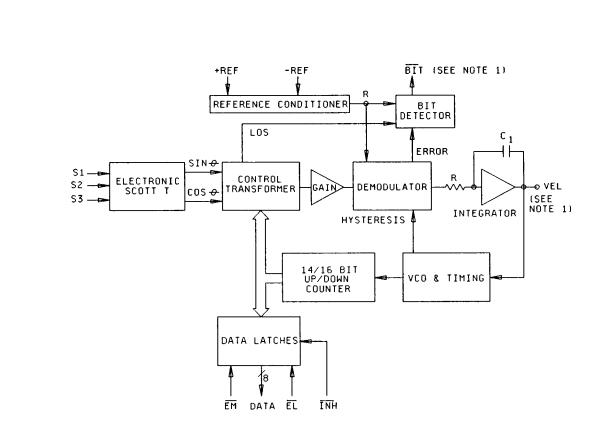
NOTE:  $\overline{\text{BIT}}$  is not connected on device types 01, 03, 05, 07, 09 and 11. VEL is not connected on device types 02, 04, 06, 08, 10, and 12.
