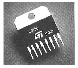
One alternative, widely used in simple power ICs, is to use thick (250um) aluminum wires. However, a thick aluminum bonding wire needs a large bonding pad on the die. In a simple device like a 3-terminal voltage regulator this is not a problem because there are few such pads, but for more complex ICs with eight or more connections the wasted silicon area would be excessive.
