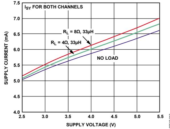
Figure 13. Supply Current vs. Supply Voltage, No Load
