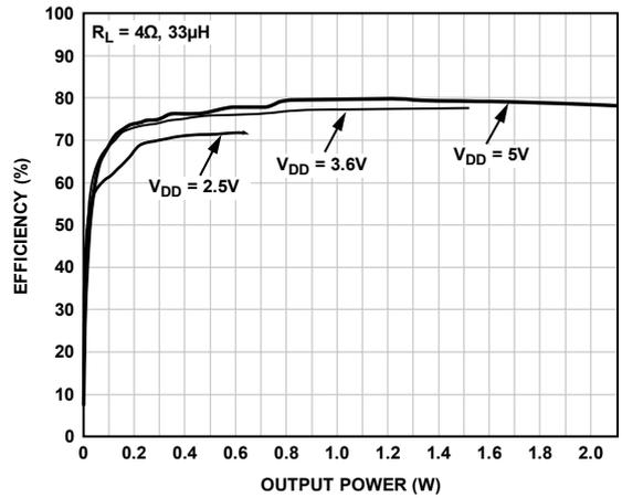
Figure 19. Efficiency vs. Output Power into  $4\ \Omega$
