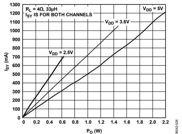
Figure 26. Supply Current vs. Output Power into  $4\Omega$
