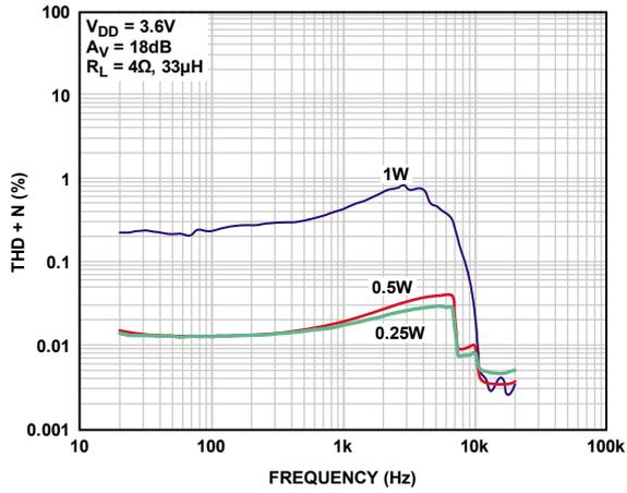
Figure 10. THD + N vs. Frequency,  $V_{DD} = 3.6\text{ V}$ ,  $R_L = 4\ \Omega$ ,  $A_V = 18\text{ dB}$
