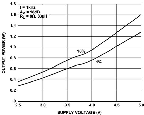
Figure 17. Maximum Output Power vs. Supply Voltage,  $R_L = 8\ \Omega$ ,  $A_V = 18\ \text{dB}$
