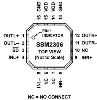
Figure 2. Pin Configuration
