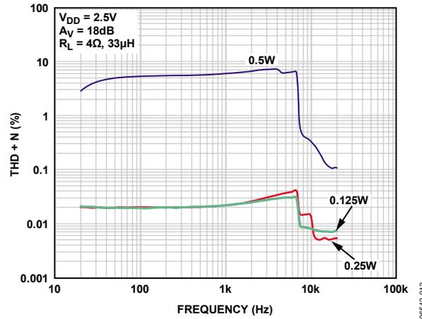
Figure 12. THD + N vs. Frequency,  $V_{DD} = 2.5\text{ V}$ ,  $R_L = 4\ \Omega$ ,  $A_V = 18\text{ dB}$
