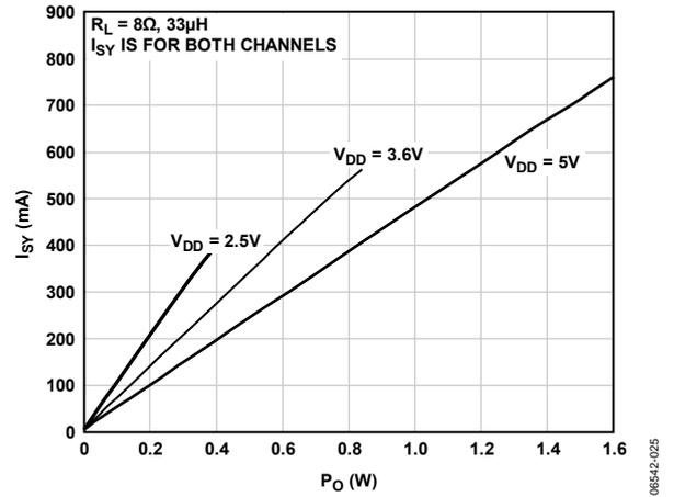
Figure 25. Supply Current vs. Output Power into  $8\Omega$
