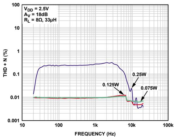
Figure 11. THD + N vs. Frequency,  $V_{DD} = 2.5\text{ V}$ ,  $R_L = 8\ \Omega$ ,  $A_V = 18\text{ dB}$
