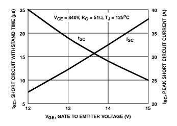
FIGURE 4. SHORT CIRCUIT WITHSTAND TIME
