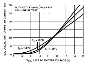
FIGURE 13. TRANSFER CHARACTERISTIC
