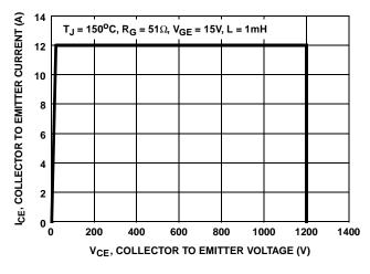
FIGURE 2. MINIMUM SWITCHING SAFE OPERATING AREA
