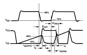
FIGURE 19. SWITCHING TEST WAVEFORMS
