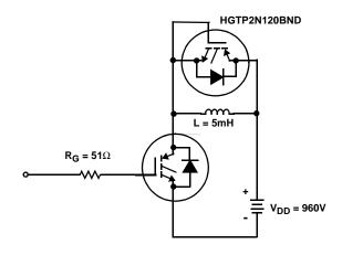
FIGURE 18. INDUCTIVE SWITCHING TEST CIRCUIT
