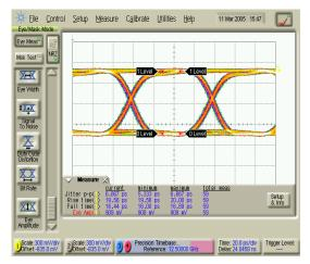
**Die Measurement** VEE: -5V Input Data Rate **12.5 Gb/s** Single ended Data Input (0/-500mV)
