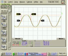
**Die Measurement** VEE: -5V Input Clock Frequency **10.7GHz** Differential Data Input (0/-500mV)
