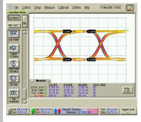
**Die Measurement** VEE: -5V Input Data Rate **10.7 Gb/s** Single ended Data Input (0/-500mV)
