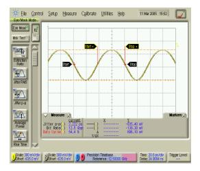
**Die Measurement** VEE: -5V Input Clock Frequency **12.5GHz** Single ended Data Input (0/-500mV)
