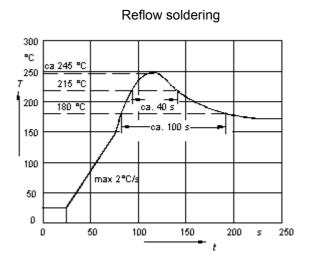
As far as possible, the components shall be employed within 12 months. They should be left in their original packings to avoid soldering problems due to oxidized contacts. Storage temperature: –25 to 45 °C. Relative humidity: <75 % annual average, <95 % on max. 30 days in a year.
