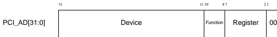
Bit 31 of the 36-bit physical address is a zero and causes the PCI controller to emit “00” on PCI\_AD[1:0]. During the address phase, only one bit is permitted to be set in the Device number field. The single “1” bit denotes the IDSEL of a PCI target device for the configuration cycle. A total of 20 target devices is supported. The following table enumerates the 20 possible configuration spaces.
