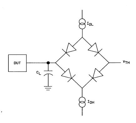
NOTE: Test conditions shall be as follows:  $C_L = 30 \text{ pF}$ ,  $V_{TH} = 1.5 \text{ V}$ ,  $I_{OL} = 8 \text{ mA}$ ,  $I_{OH} = -2 \text{ mA}$  for all ac parameters with the exception of  $t_{ENA}/t_{DIS}$ . For  $t_{ENA}/t_{DIS}$ , test conditions shall be:  $C_L = 30 \text{ pF}$ ,  $V_{TH} = 10 \text{ mA}$ .
