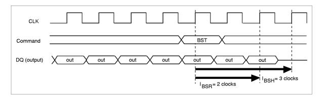
Burst stop command at burst write: The burst stop command (BST command) is used to stop data input during a full-page burst write. No data is written in the same clock as the BST command, and in subsequent clocks. In addition, the BST command is only valid during full-page burst mode, and is illegal with burst lengths of 1, 2, 4 and 8. And an interval of  $t_{DPL}$  is required between last data-in and the next precharge command.
