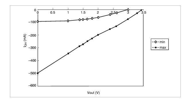
**DC Characteristics** (Ta = 0 to 70°C,  $V_{CC}$ ,  $V_{CC}Q = 3.3 \text{ V} \pm 0.3 \text{ V}$ ,  $V_{SS}$ ,  $V_{SS}Q = 0 \text{ V}$ ) (HM5212165D)
