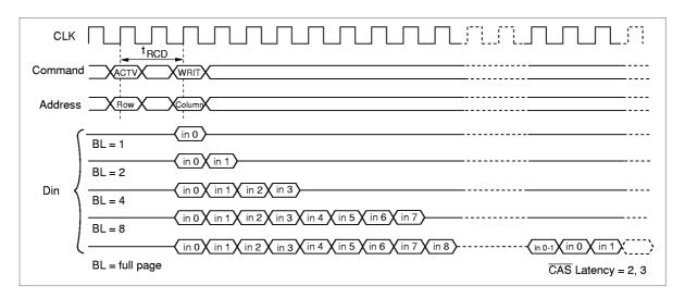
**2. Single write:** A single write operation is enabled by setting OPCODE (A9, A8) to (1, 0). In a single write operation, data is only written to the column address (AY0 to AY8; HM5212165D, AY0 to AY9; HM5212805D) and the bank select address (A12/A13) specified by the write command set cycle without regard to the burst length setting. (The latency of data input is 0 clock).
