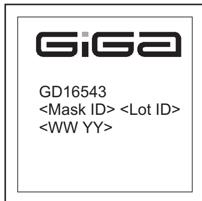
Figure 12. Device Marking, (Top - 48 pin and Bottom - 40 pin)
