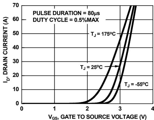
Figure 5. Transfer Characteristics
