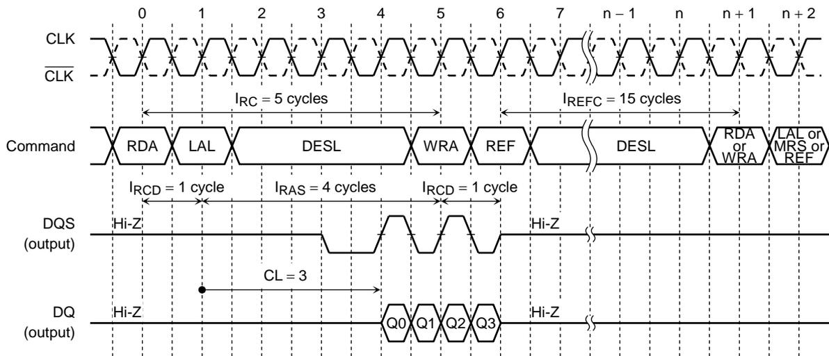
Note: In case of CL = 3, IREFC must meet 15 clock cycles.
