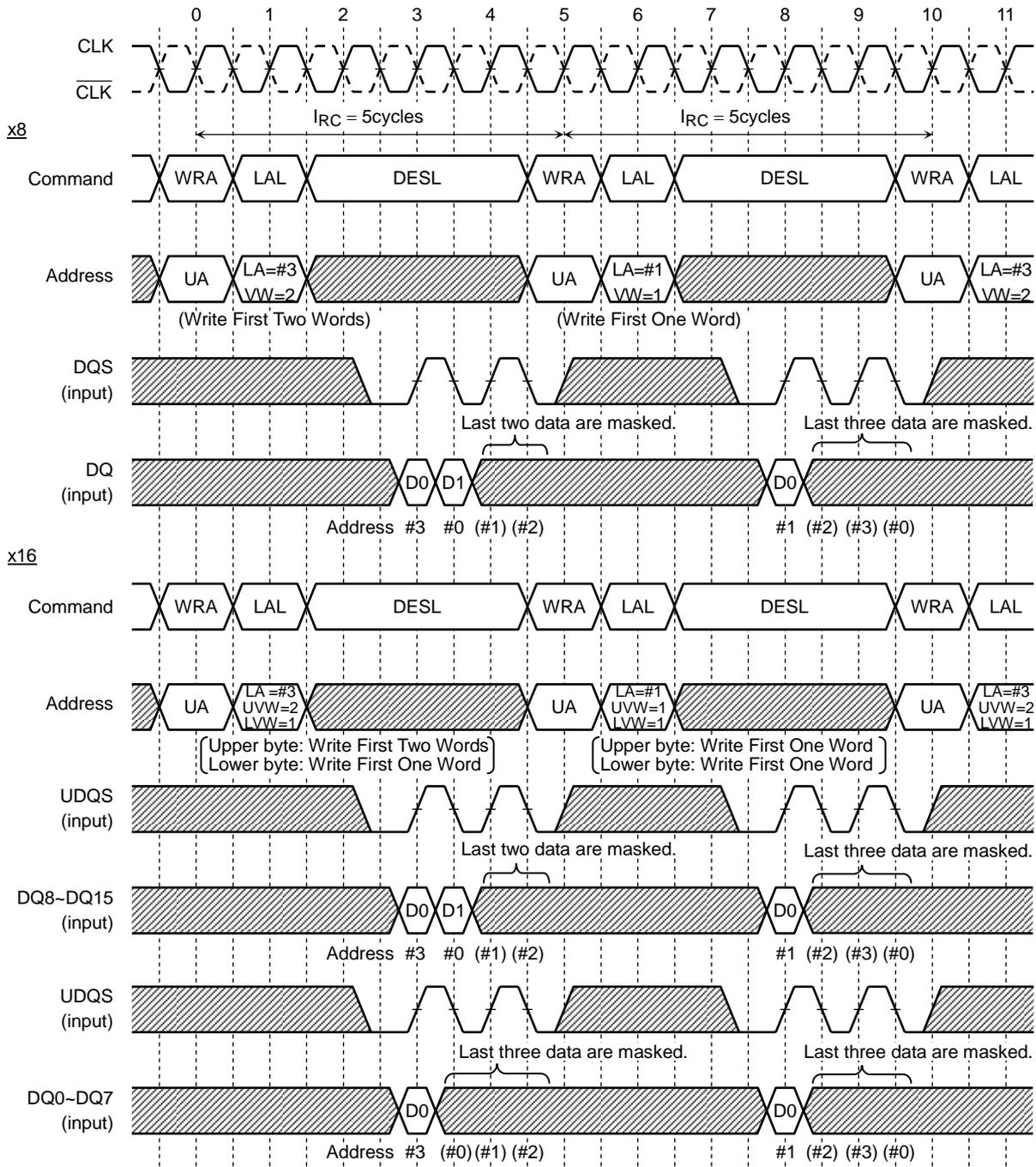
Note: DQS input must be continued till end of burst count even if some of later data is masked. Refer to "VW Truth Table".
