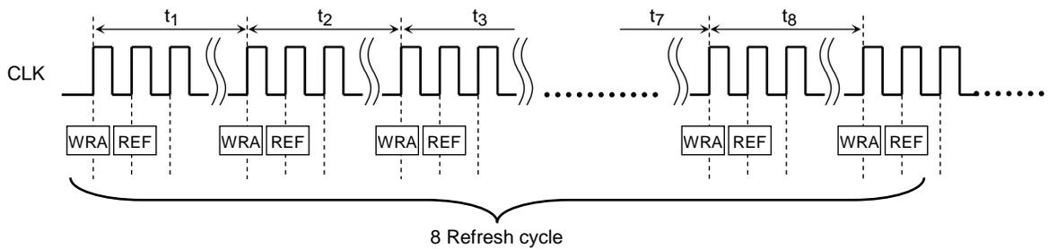
$$t_{REFI} = \frac{\text{Total time of 8 Refresh cycle}}{8} = \frac{t_1 + t_2 + t_3 + t_4 + t_5 + t_6 + t_7 + t_8}{8}$$
