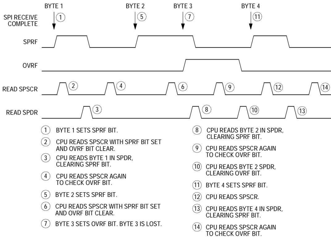
Figure 17-7. Clearing SPRF When OVRF Interrupt Is Not Enabled
