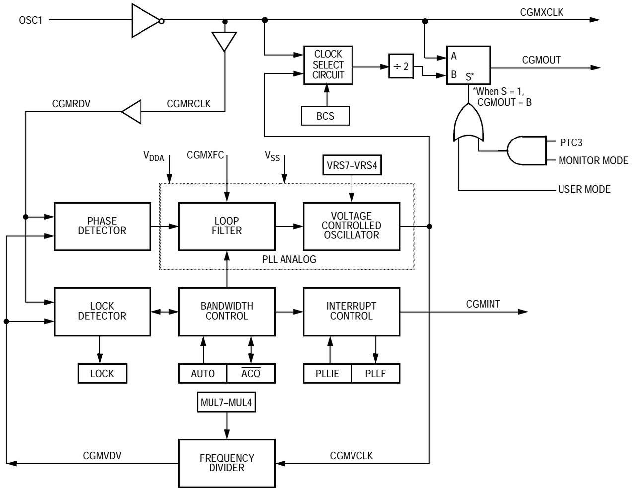
**Figure 8-1. CGM Block Diagram**
