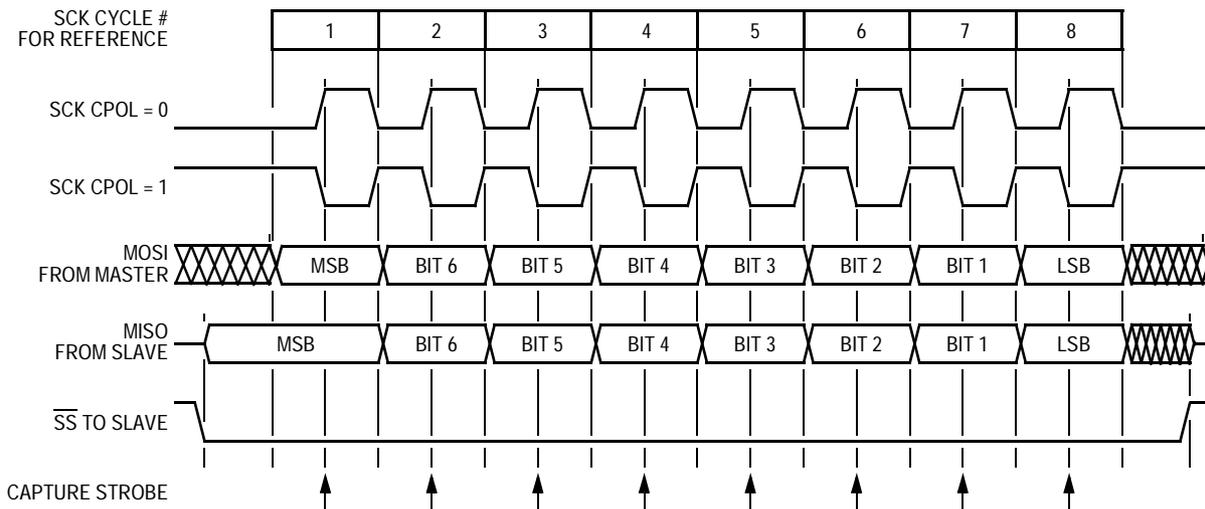
Figure 17-3. Transmission Format (CPHA = 0)
