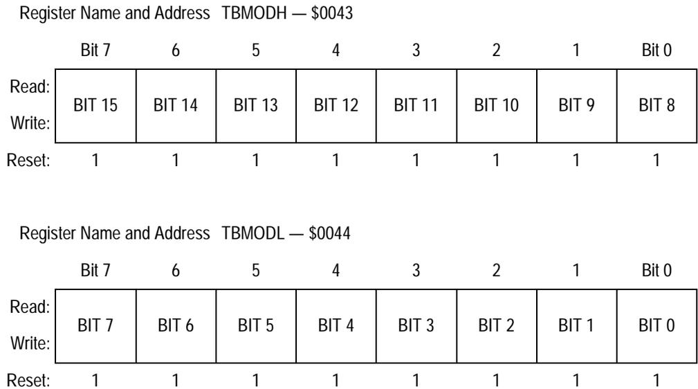
Figure 19-6. TIMB Counter Modulo Registers (TBMODH and TBMODL)
