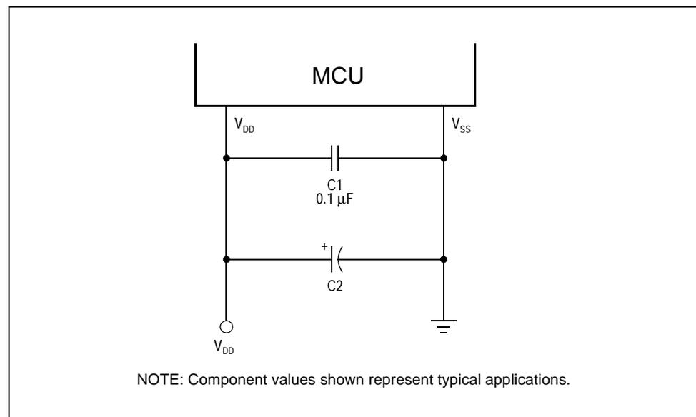
$V_{SS}$  is also the ground for the port output buffers and the ground return for the serial clock in the Serial Peripheral Interface module (SPI). See [Section 17. Serial Peripheral Interface \(SPI\)](#).
