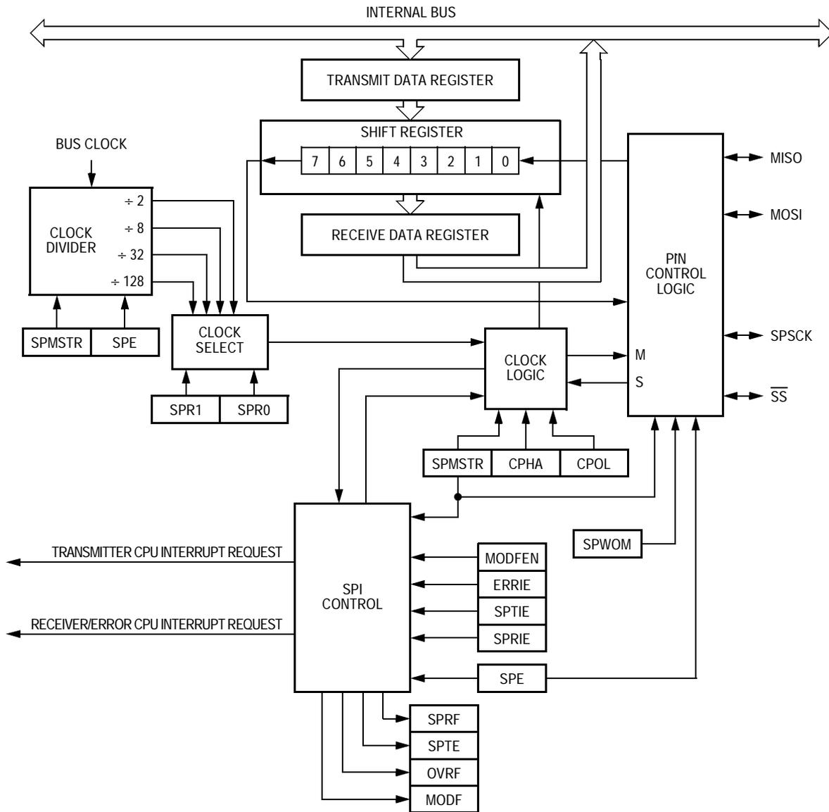
Figure 17-1. SPI Module Block Diagram
