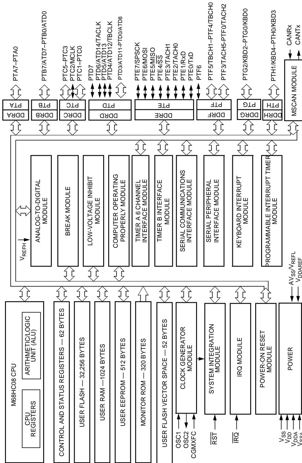
Figure 1-1. MCU Block Diagram for the MC68HC908AZ32A
