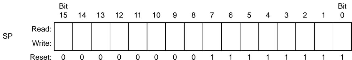
**NOTE:** The location of the stack is arbitrary and may be relocated anywhere in RAM. Moving the SP out of page zero (\$0000 to \$00FF) frees direct address (page zero) space. For correct operation, the stack pointer must point only to RAM locations.
