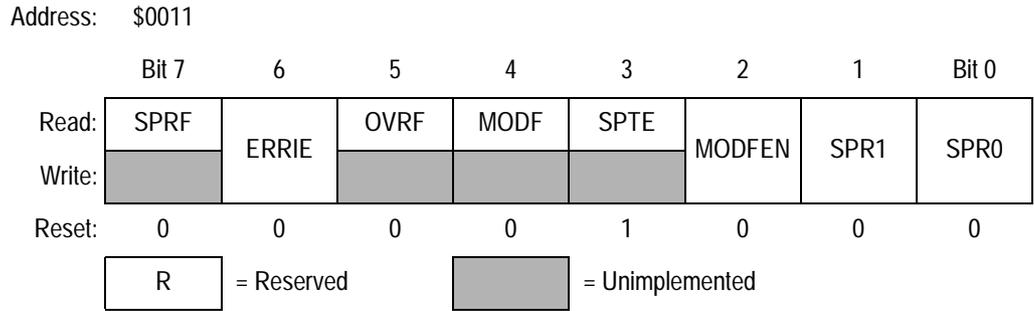
**Figure 17-12. SPI Status and Control Register (SPSCR)**
