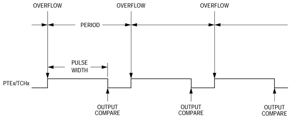
Figure 18-3. PWM Period and Pulse Width
