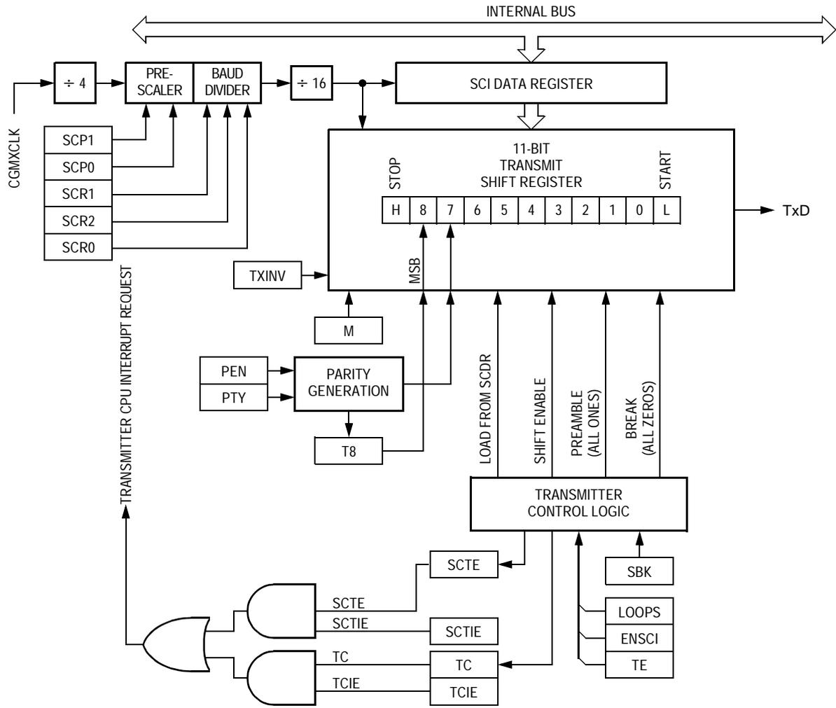
Figure 16-4. SCI Transmitter
