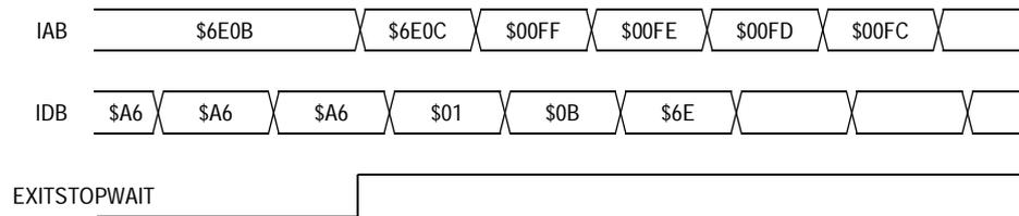
NOTE: EXITSTOPWAIT =  $\overline{\text{RST}}$  pin OR CPU interrupt OR break interrupt
