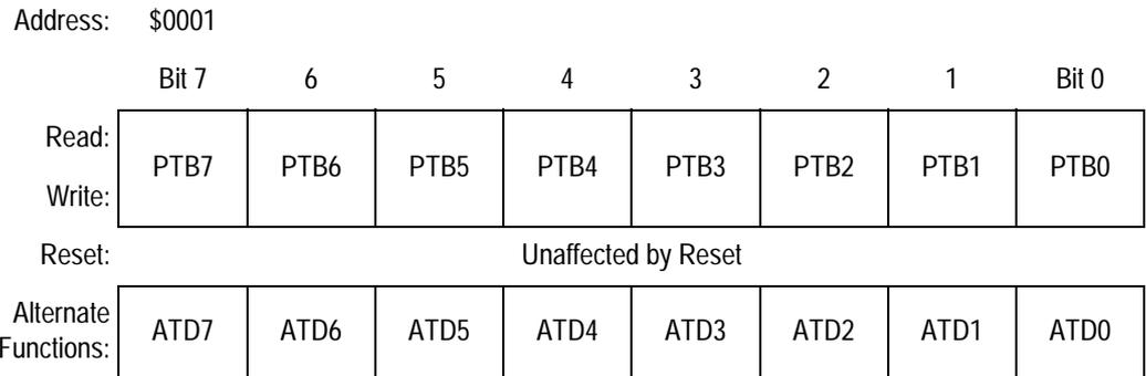
Figure 23-5. Port B Data Register (PTB)
