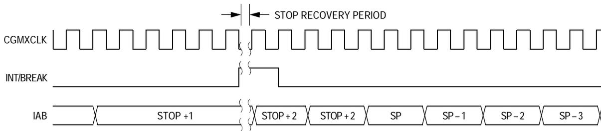
**Figure 7-16. Stop Mode Recovery from Interrupt or Break**
