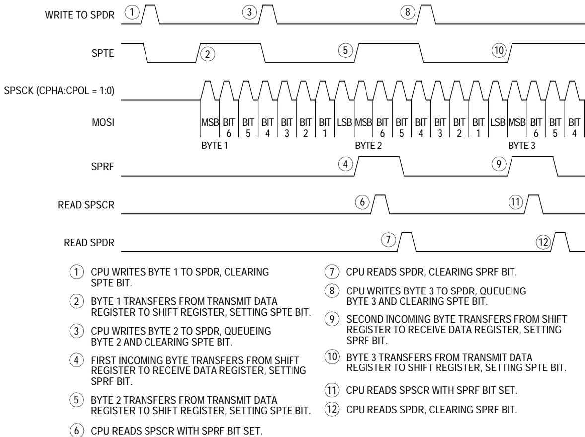
Figure 17-9. SPRF/SPTF CPU Interrupt Timing
