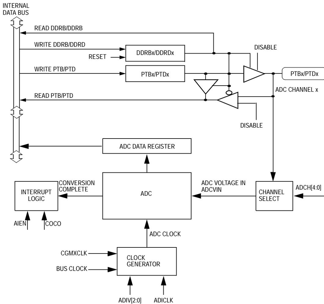
Figure 21-1. ADC Block Diagram
