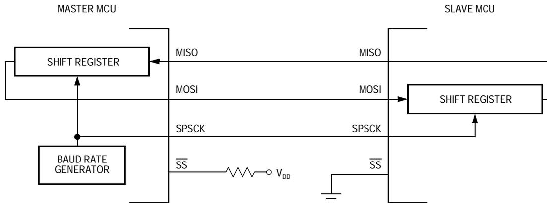
Figure 17-2. Full-Duplex Master-Slave Connections
