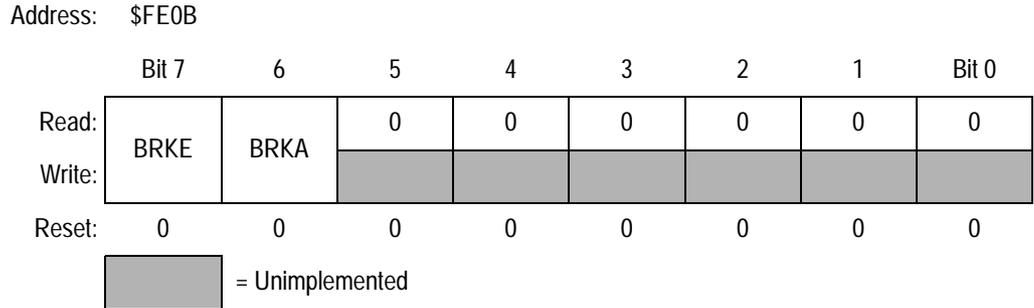
**Figure 11-3. Break Status and Control Register (BSCR)**
