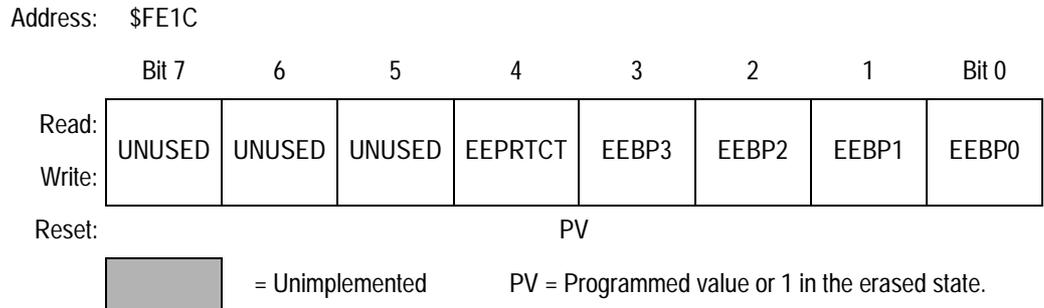
**Figure 5-4. EEPROM Nonvolatile Register (EENVR)**
