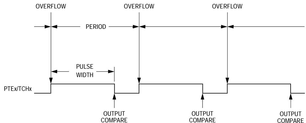
**Figure 19-3. PWM Period and Pulse Width**
