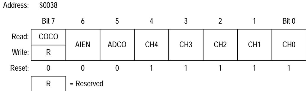
**Figure 21-2. ADC Status and Control Register (ADSCR)**
