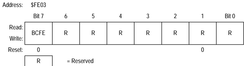
**Figure 7-19. SIM Break Flag Control Register (SBFCR)**
