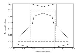
Figure-2 E1 Waveform Template Diagram
