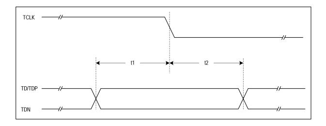
Figure-17 Transmit System Interface Timing
