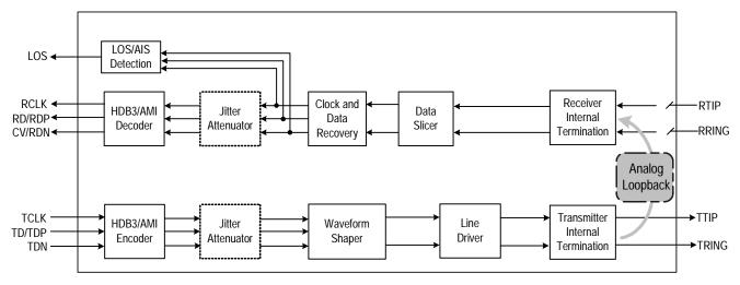
Figure-10 Analog Loopback
