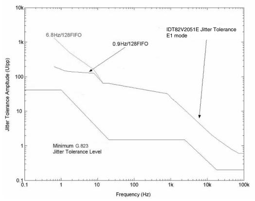
Figure-19 E1 Jitter Tolerance Performance
