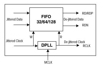
Figure-8 Jitter Attenuator
