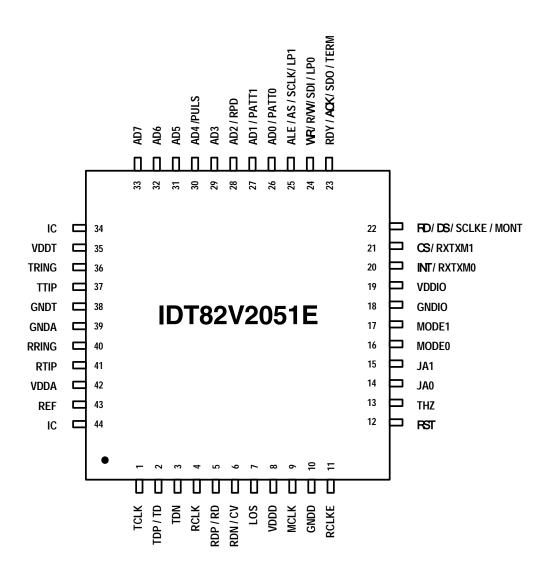
Figure-1 IDT82V2051E TQFP44 Package Pin Assignment
