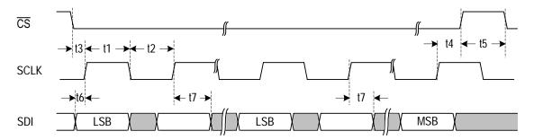
Figure-21 Serial Interface Write Timing
