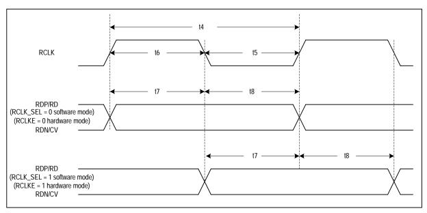
Figure-18 Receive System Interface Timing
