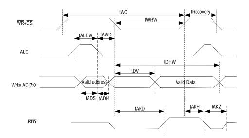
Figure-27 Multiplexed Intel Write Timing
