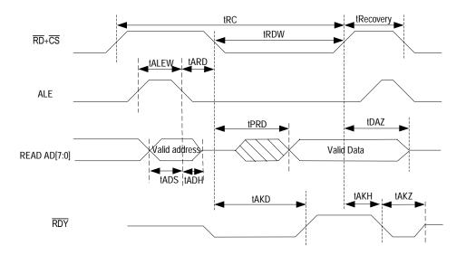
Figure-26 Multiplexed Intel Read Timing
