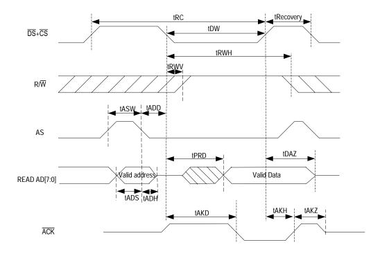
Figure-24 Multiplexed Motorola Read Timing
