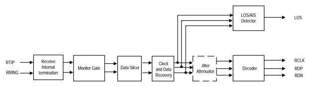
Figure-4 Receive Path Function Block Diagram
