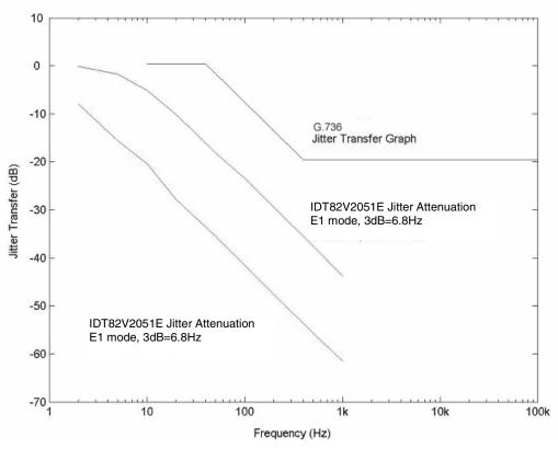
Figure-20 E1 Jitter Transfer Performance
