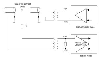
Figure-7 Monitor Transmit Line in Another Chip
