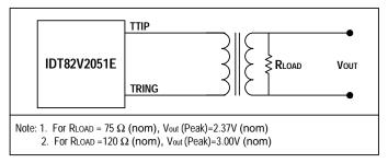
Figure-3 E1 Pulse Template Test Circuit
