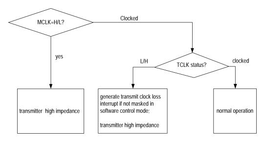
Figure-15 TCLK Operation Flowchart
