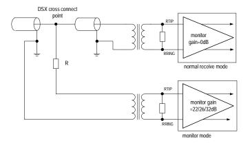
Figure-6 Monitoring Receive Line in Another Chip
