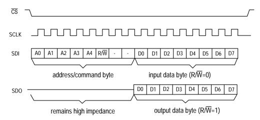
Figure-16 Serial Microcontroller Interface Function Timing
