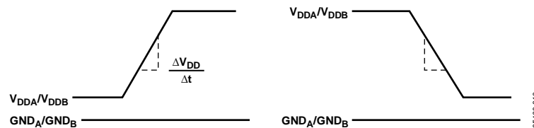
Figure 13. Transient Immunity Waveforms—Output Supplies
