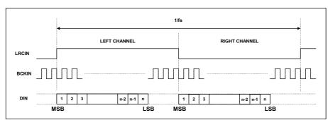
Figure 8 Left Justified Mode Timing Diagram
