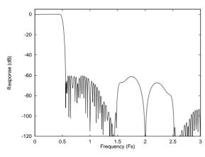
Figure 17 DAC Digital Filter Frequency Response -44.1, 48 and 96kHz
