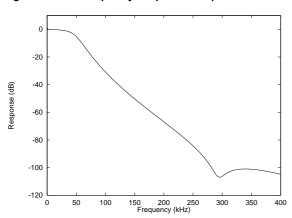
Figure 28 DSD Frequency Response - no post filter
