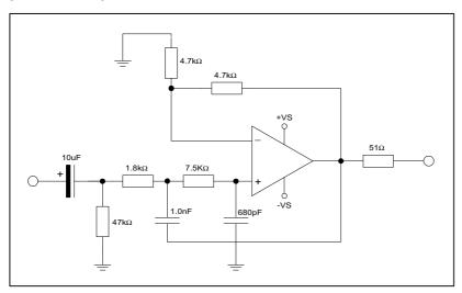
Figure 35 Recommended Low Pass Filter (Optional)
