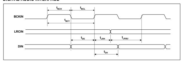
Figure 2 Digital Audio Data Timing
