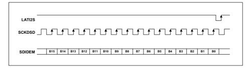
Figure 15 3-Wire Serial Interface
