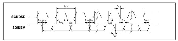
Figure 7 Program Register Input Timing - 2-Wire Serial Control Mode
