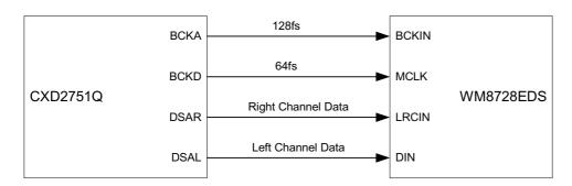
Figure 34 Biphase Mode Connection Diagram
