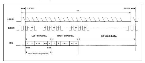
Figure 11 DSP Early Mode Timing Diagram
