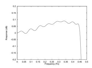
Figure 18 DAC Digital Filter Ripple -44.1, 48 and 96kHz
