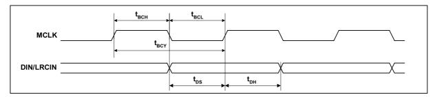
Figure 3 Normal DSD timing requirements
