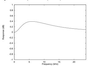
Figure 25 De-Emphasis Frequency Response (48kHz)
