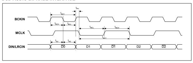
Figure 5 Biphase DSD Timing Requirements
