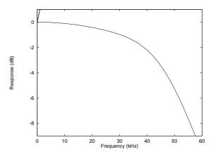
Figure 29 DSD frequency response - 4th order post filter
