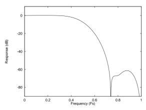
Figure 19 DAC Digital Filter Frequency Response -192kHz
