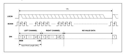
Figure 12 DSP Late Mode Timing Diagram
