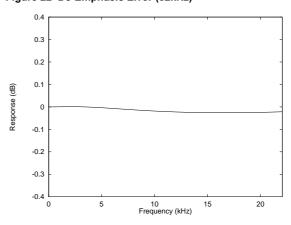
Figure 23 De-Emphasis Frequency Response (44.1kHz)
