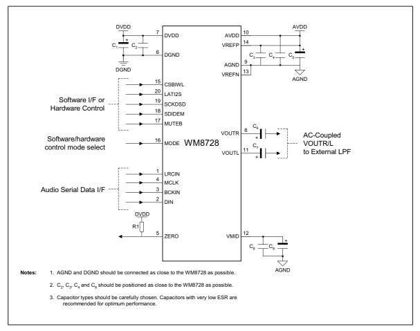
Figure 31 External Components Diagram
