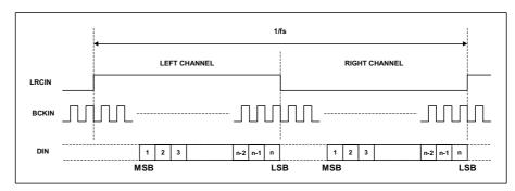
Figure 9 Right Justified Mode Timing Diagram
