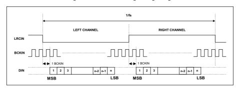
Figure 10 I<sup>2</sup>S Mode Timing Diagram
