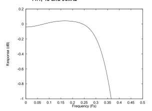
Figure 20 DAC Digital Filter Ripple -192kHz
