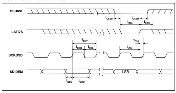
Figure 6 Program Register Input Timing - 3-Wire Serial Control Mode
