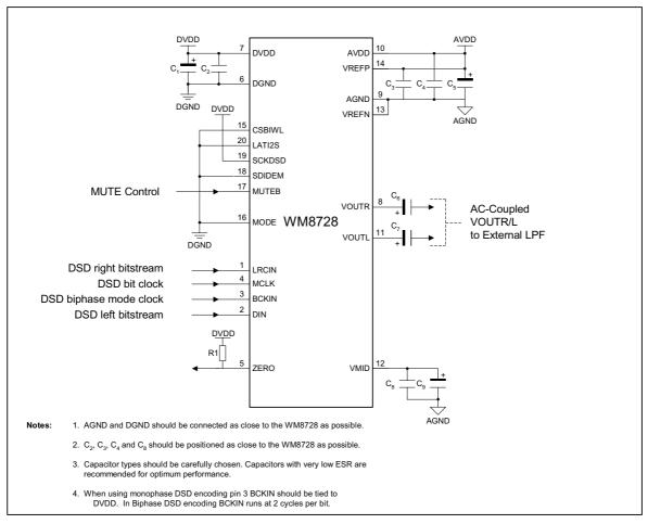
Figure 32 External Connections for DSD Applications
