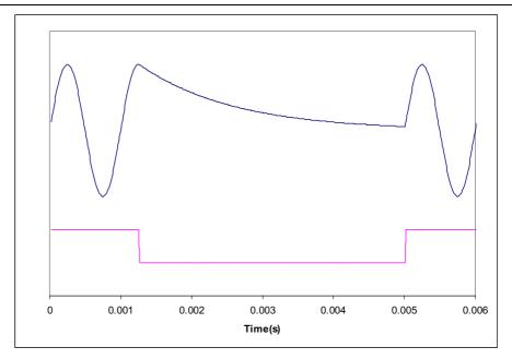
Figure 13 Application and Release of Soft Mute
