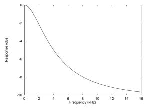
Figure 21 De-Emphasis Frequency Response (32kHz)
