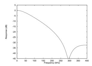
Figure 27 DSD Frequency Response - no post filter
