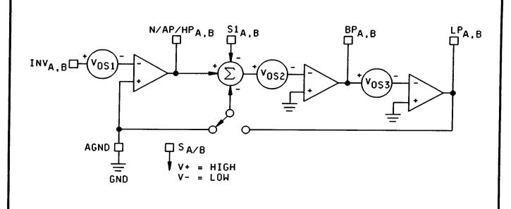
FIGURE 4. Equivalent input offsets of 1/2 filter building block.
