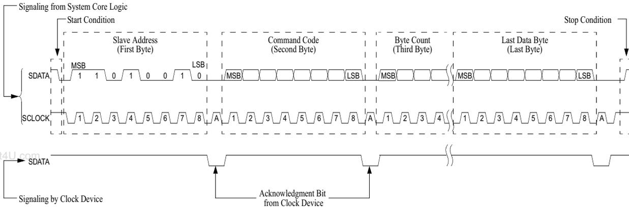
**Figure 4. Serial Data Bus Write Sequence**
