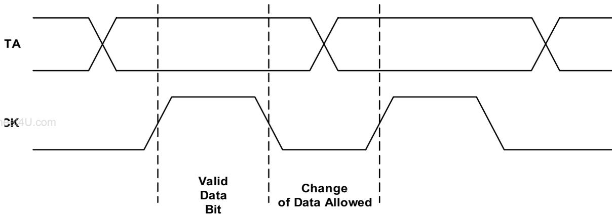
Figure 2. Serial Data Bus Valid Data Bit
