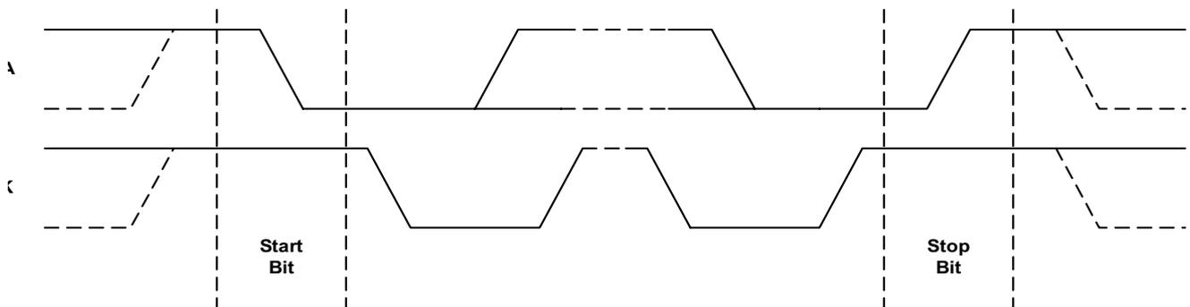
Figure 3. Serial Data Bus Start and Stop Bit
