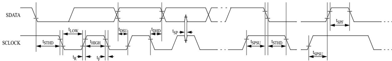
**Figure 5. Serial Data Bus Timing Diagrams**
