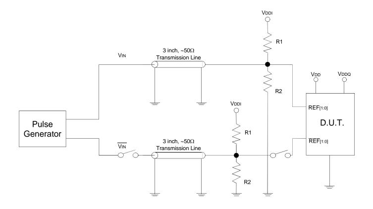
Test Circuit for Differential Input<sup>(1)</sup>
