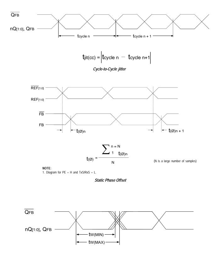
$t_{JIT(DUTY)} = |t_{W(MAX)} - t_{W(MIN)}|$
