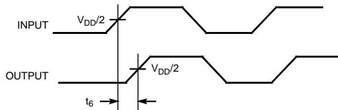
**Figure 7. Device-Device Skew**
