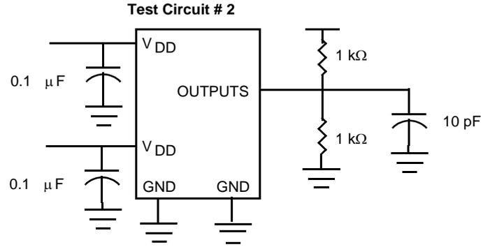
For parameter  $t_b$  (output slew rate) on -1H devices
