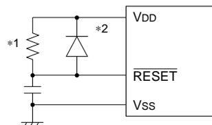
\*1 When the built-in pull-up resistor is not used.
