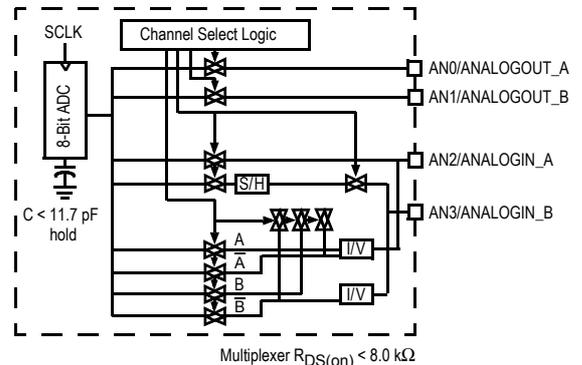
**Figure 14. A/D Converter Input Structure**
