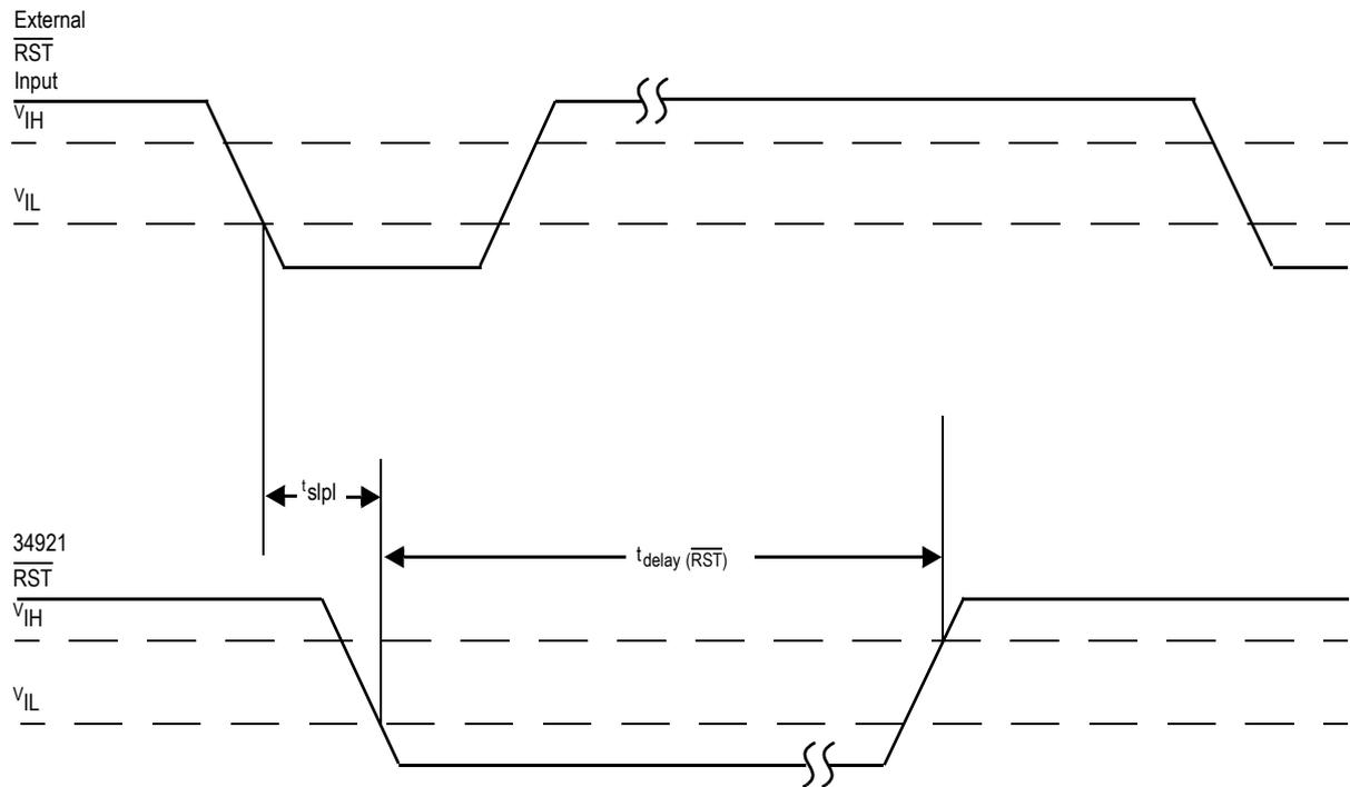
**Figure 6.  $\overline{\text{RST}}$  Timing**
