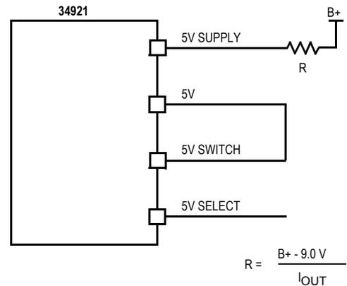
**Figure 9. 5.0 V Linear Regulator Mode**
