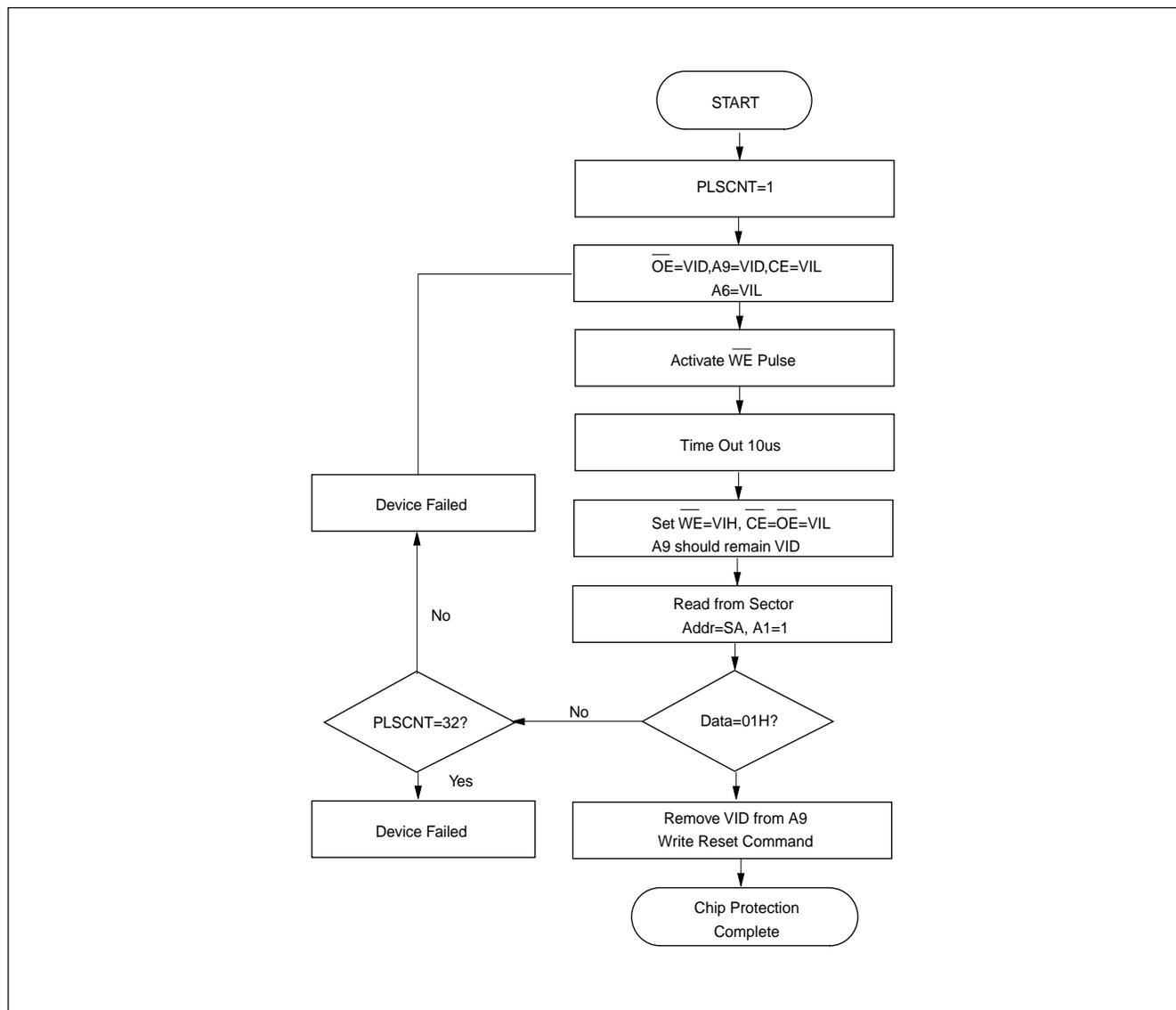
**CHIP UNPROTECTION ALGORITHM FOR SYSTEM WITH 12V**
