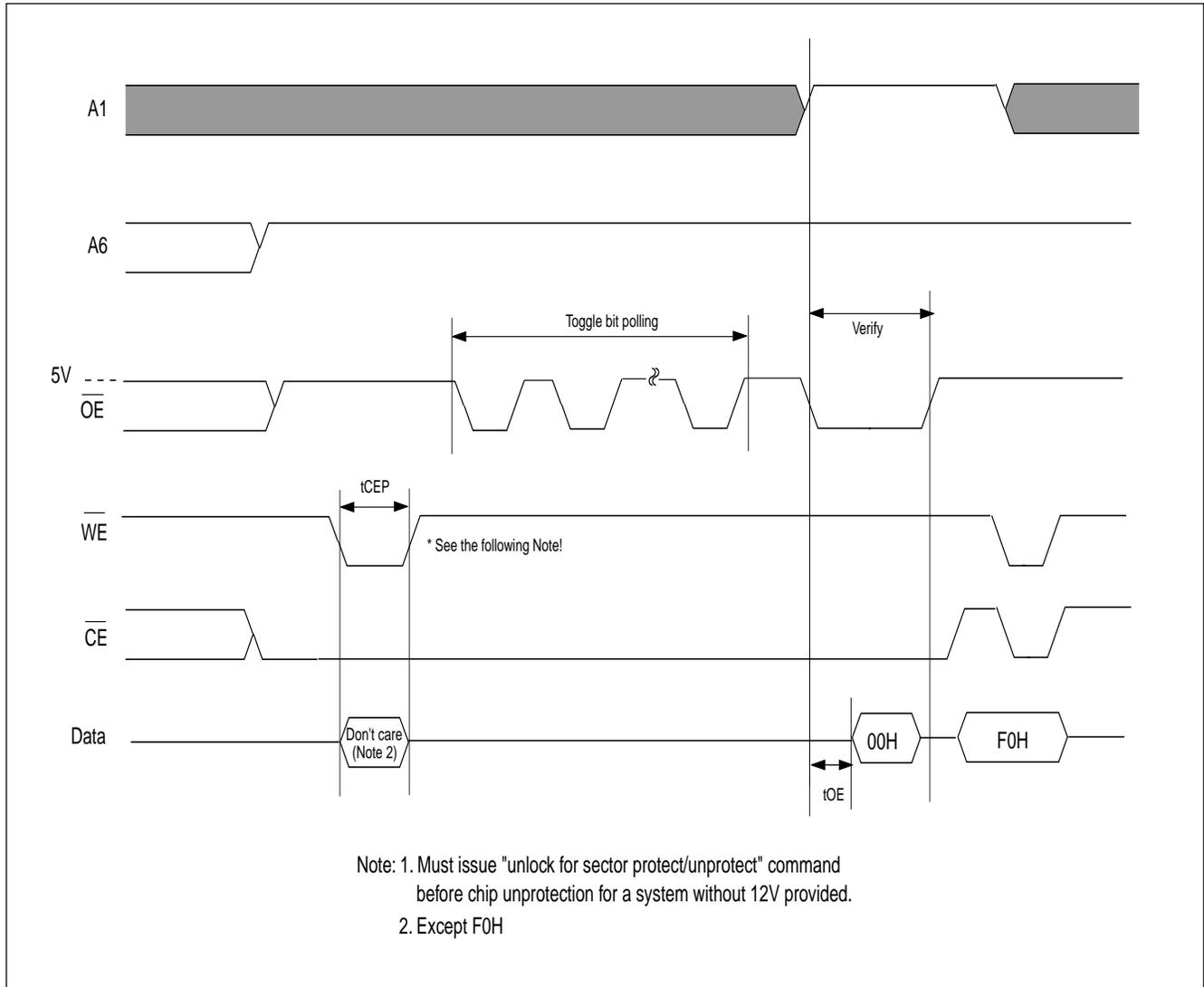
**CHIP PROTECTION ALGORITHM FOR SYSTEM WITHOUT 12V**
