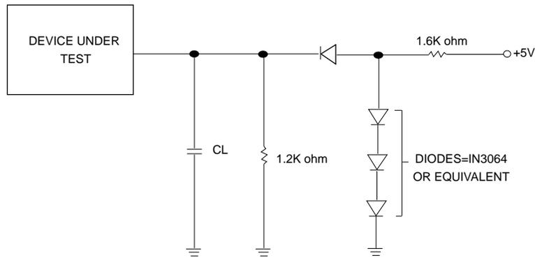
CL=100pF Including jig capacitance for 29F001T/B-70, 29F001T/B-90, 29F001T/B-12
