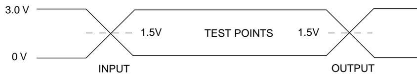
AC TESTING: Inputs are driven at 3.0V for a logic "1" and 0V for a logic "0".
