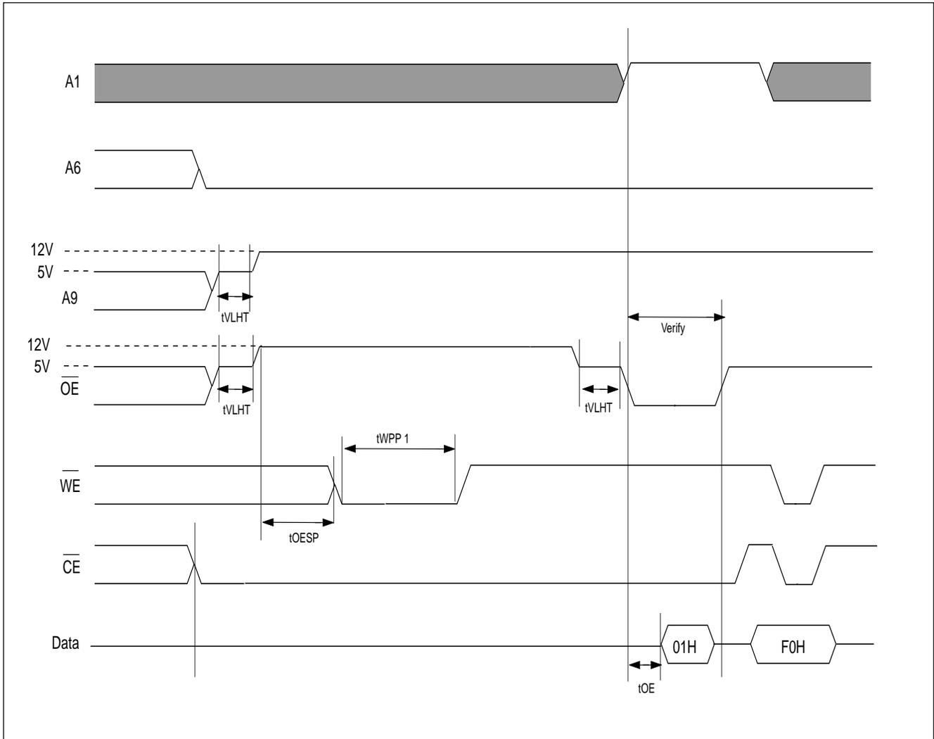
**TIMING WAVEFORM FOR CHIP UNPROTECTION FOR SYSTEM WITH 12V**
