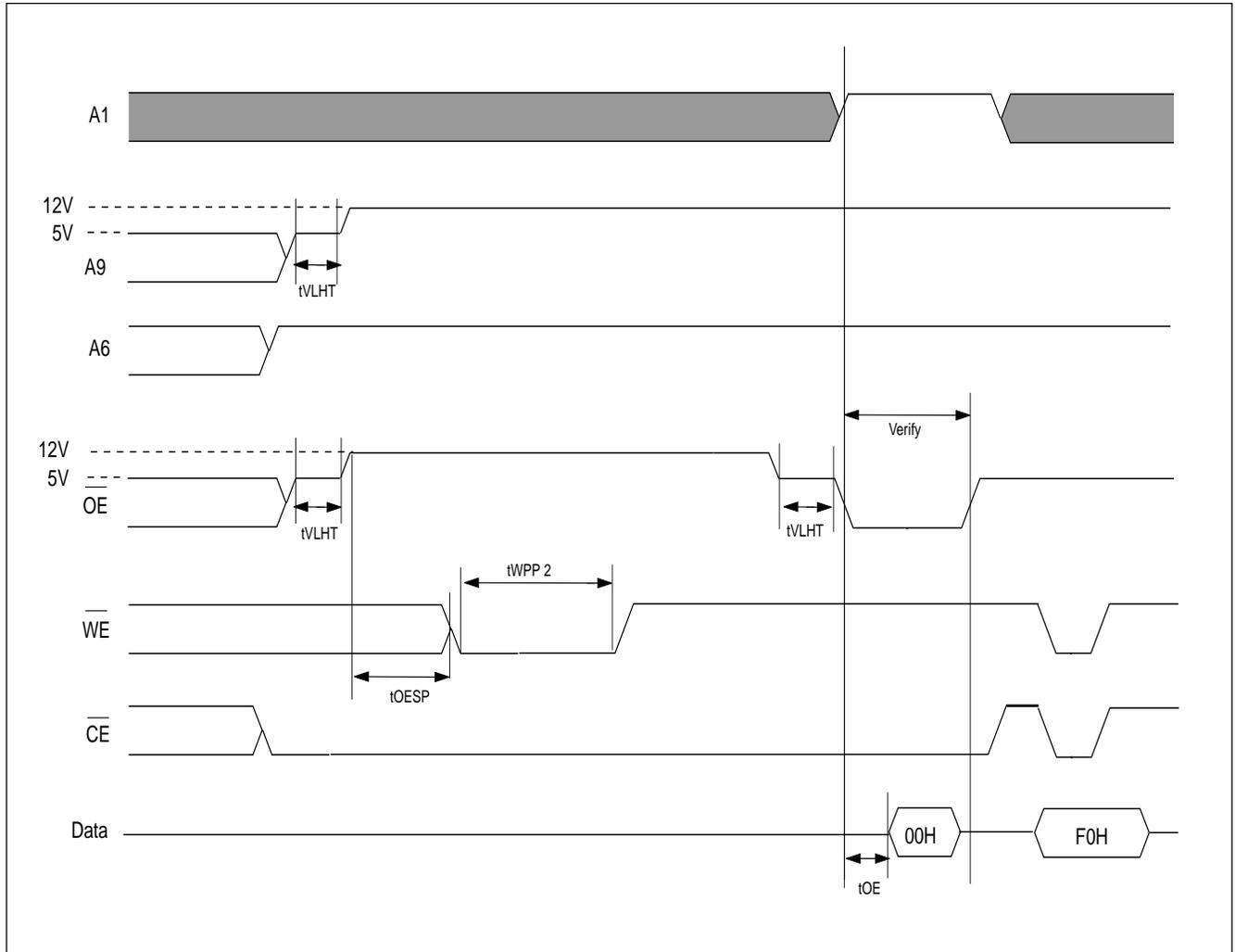
**CHIP PROTECTION ALGORITHM FOR SYSTEM WITH 12V**
