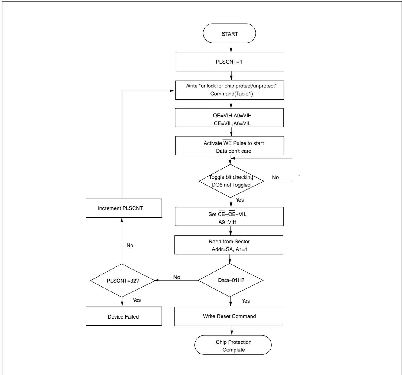
**CHIP UNPROTECTION ALGORITHM FOR SYSTEM WITHOUT 12V**
