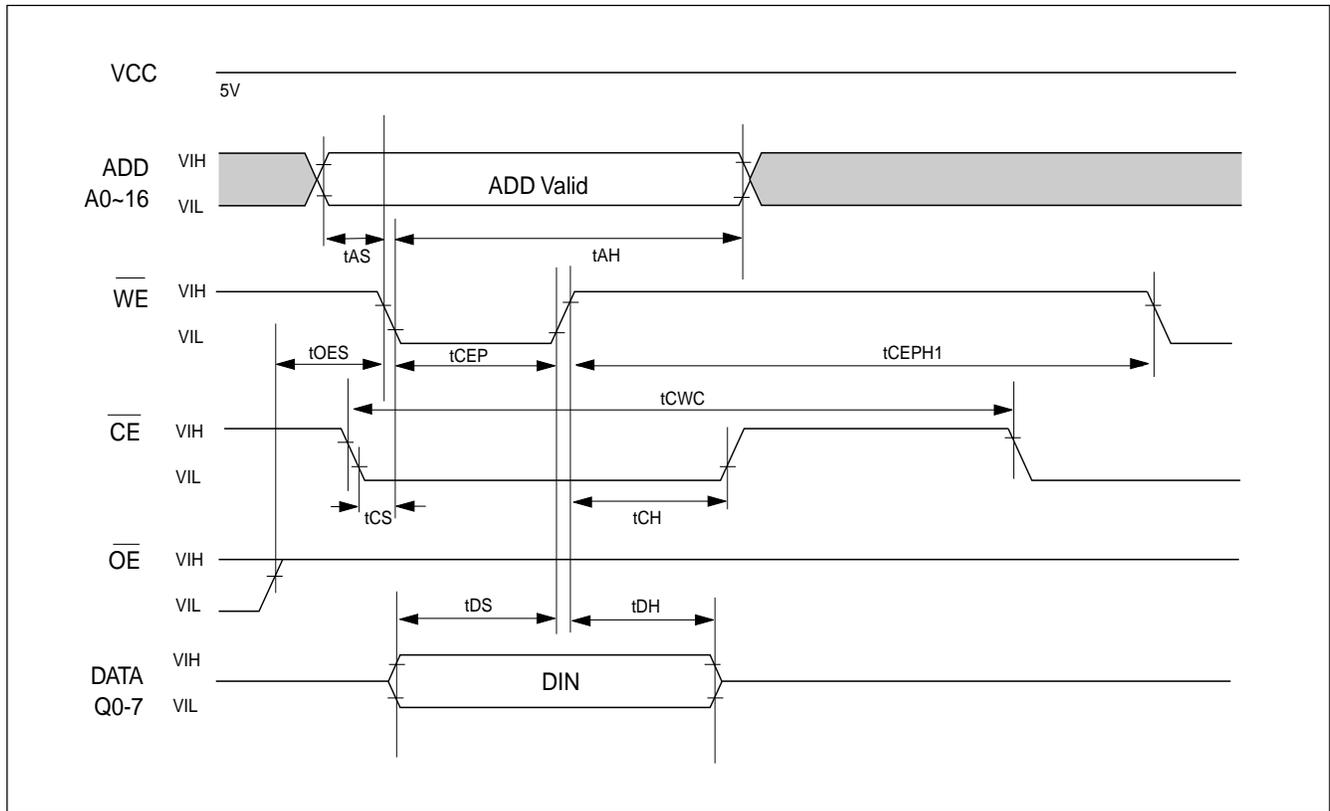
**AUTOMATIC PROGRAMMING TIMING WAVEFORM**
