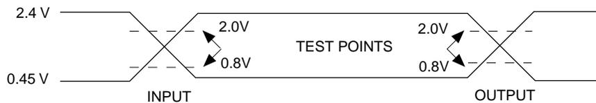
AC TESTING: Inputs are driven at 2.4V for a logic "1" and 0.45V for a logic "0".
