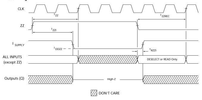
Notes: 21. Device must be deselected when entering ZZ mode. See Cycle Descriptions table for all possible signal conditions to deselect the device. 22. DQs are in High-Z when exiting ZZ sleep mode.
