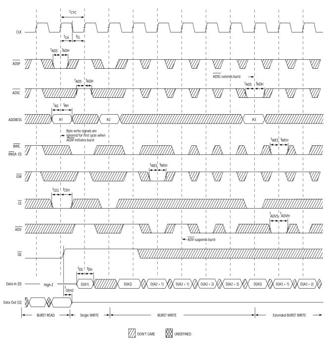
**Note:** 18. Full width Write can be initiated by either  $\overline{GW}$  LOW; or by  $\overline{GW}$  HIGH,  $\overline{BWE}$  LOW and  $\overline{BW}_{[A: D]}$  LOW.
