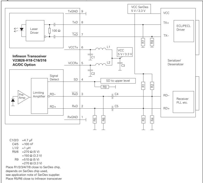
Values of R1/2/3/4 may vary as long as proper 50  $\Omega$  termination to  $V_{EE}$  or 100  $\Omega$  differential is provided. The power supply filtering is required for good EMI performance. Use short tracks from the inductor L1/L2 to the module  $V_{CC}Rx/V_{CC}Tx.$  We strongly recommend a GND plane under the module for getting good EMI performance.
