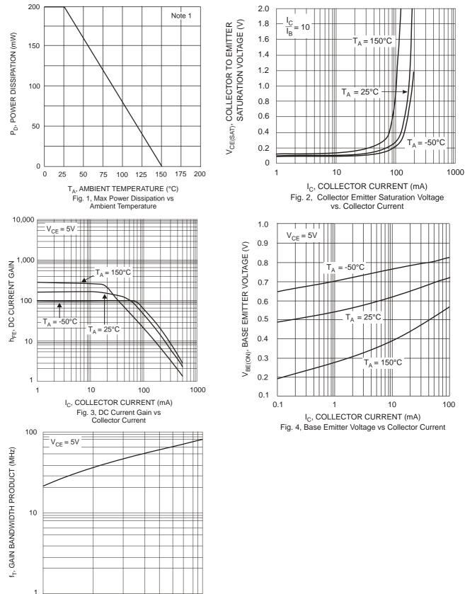
I<sub>C</sub>, COLLECTOR CURRENT (mA) Fig. 5, Gain Bandwidth Product vs Collector Current
