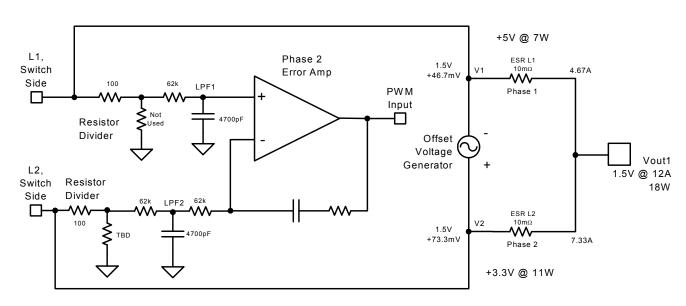
Figure 8 - LoadSHARE Using Feedback Divider Offset
