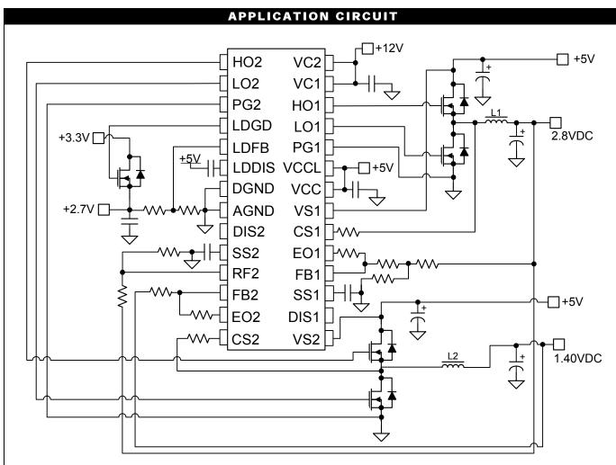
Figure 5 - Bi-Phase Operation with Phase 2 Output Tracking The Output of Phase 1.
