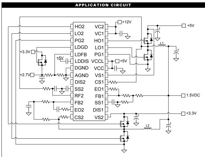
Figure 4 - Bi-Phase Operation With Phase 1 & 2 LoadSHARing From 5V & 3.3V
