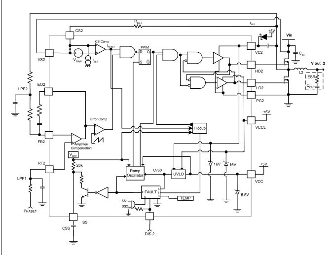
Figure 3- Block Diagram of Phase 2 Connected in LoadSHARE Mode
