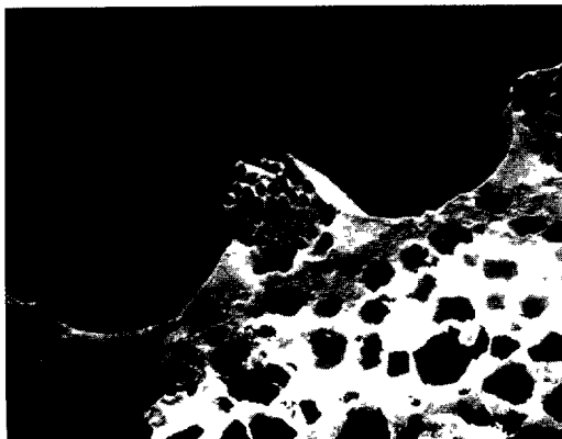
Magnified cross-section showing self-terminating conductive knitted layer detail
