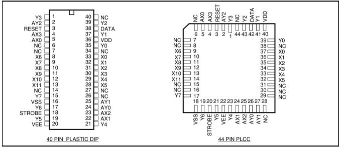
**Figure 2 - Pin Connections**
