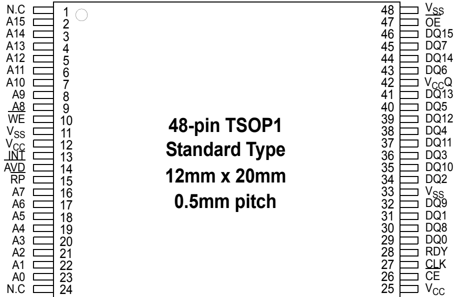
(TOP VIEW, Facing Down) TSOP1 OneNAND Chip 48pin, 12mm x 20mm, 0.5mm pitch TSOP1
