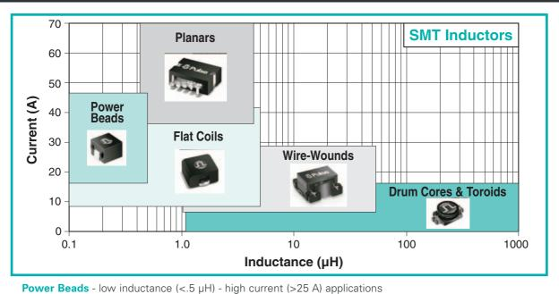
Flat Coils - mid-inductance (.5  $\mu$ H to 4  $\mu$ H) - medium current (15-30 A) applications Planars - mid-inductance (.5 μH to 4 μH) - high current (>25 A) applications Wirewound - high inductance (>5 μH) - medium current (15-30 A) applications Unshielded Drum Core Inductors - typically for lower current, portable or small power applications
