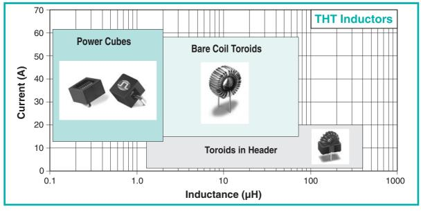
Power Cube Inductors - high-current inductors for use in low inductance applications where board space and height are critical
