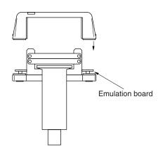
(2) Connecting emulation board (IE-789xx-NS-EM1: Probe board + I/O board) (2-board configuration)
