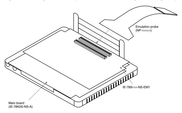
Caution The emulation probe (NP-xxxx) mounting location varies depending on the model of the I/O emulation board (IE-789xx-NS-EM1) in use. For details, refer to the IE-789xx-NS-EM1 User's Manual.
