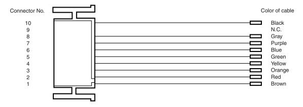
The names of the external sense probes when they are connected to EXTCN1 and EXTCN2 are as follows.
