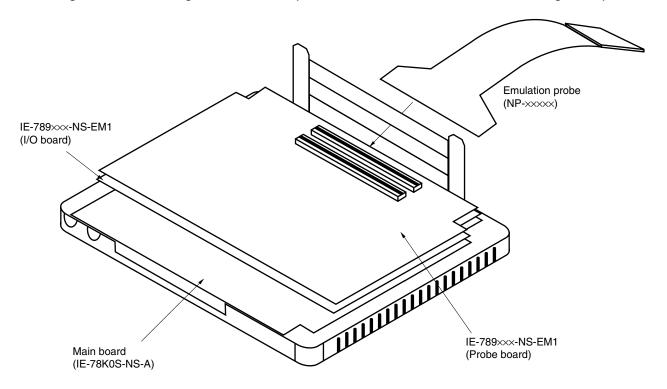
Caution The emulation probe (NP-xxxx) mounting location varies depending on the model of the I/O emulation board (IE-789xxx-NS-EM1) in use. For details, refer to the IE-789xxx-NS-EM1 User's Manual.
