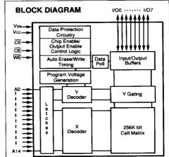
users to erase the whole memory with 5 V only power supply. Software Write Protection sets a non-volatile fuse to protect the memory from inadvertent writes.
