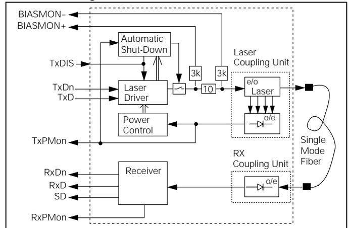
The receiver component converts the optical serial data into PECL compatible electrical data (Rx and Rx). The Signal Detect (SD, active high) shows whether an optical signal is present<sup>(1)</sup>.
