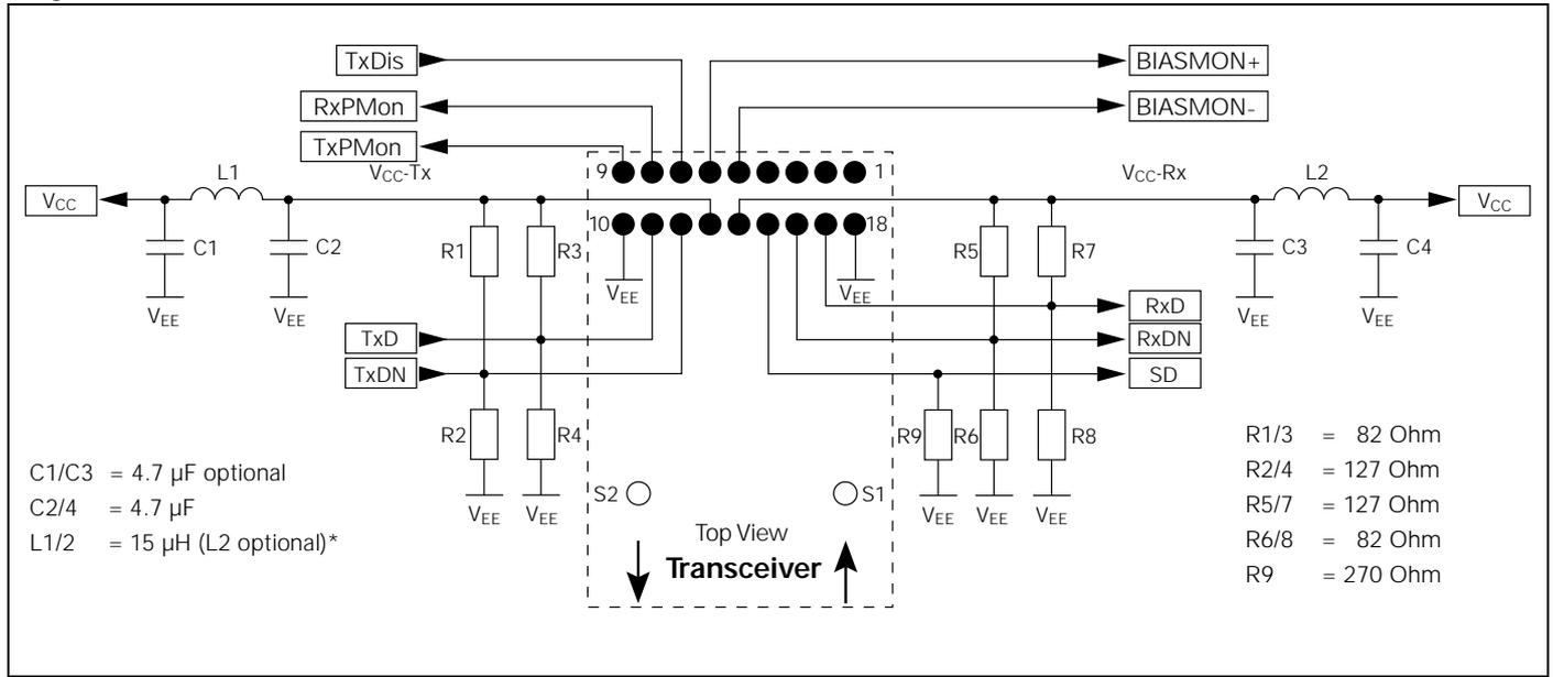
\* Recommended choke is Siemens Matsushita B78108-S1153-K or B78148-S1153-K ( $Q_{\min}=60$ , max. DC resistance = 0.6  $\Omega$ ).
