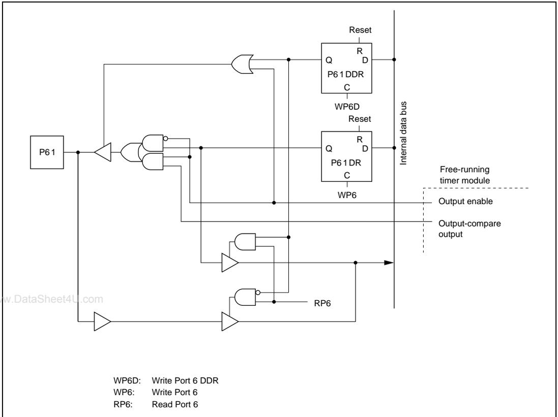
**Figure 6.6 (b) Port 6 Schematic Diagram (Pin P6<sub>1</sub>)**
