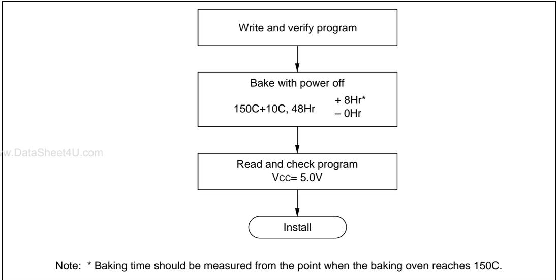
**Figure 14.7 Recommended Screening Procedure**
