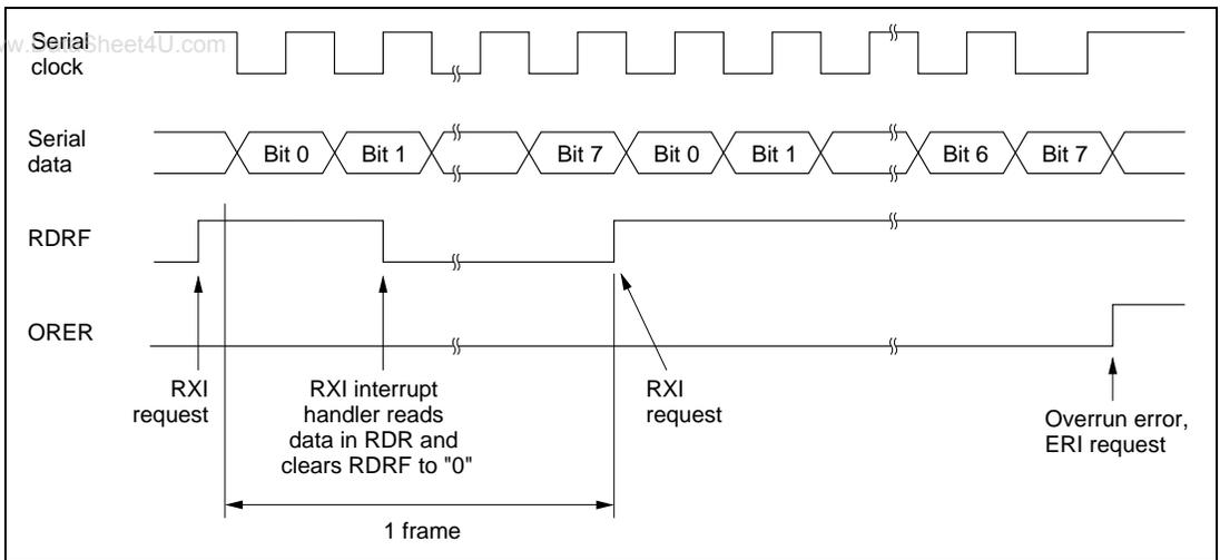
**Figure 10.16 Example of SCI Receive Operation**
