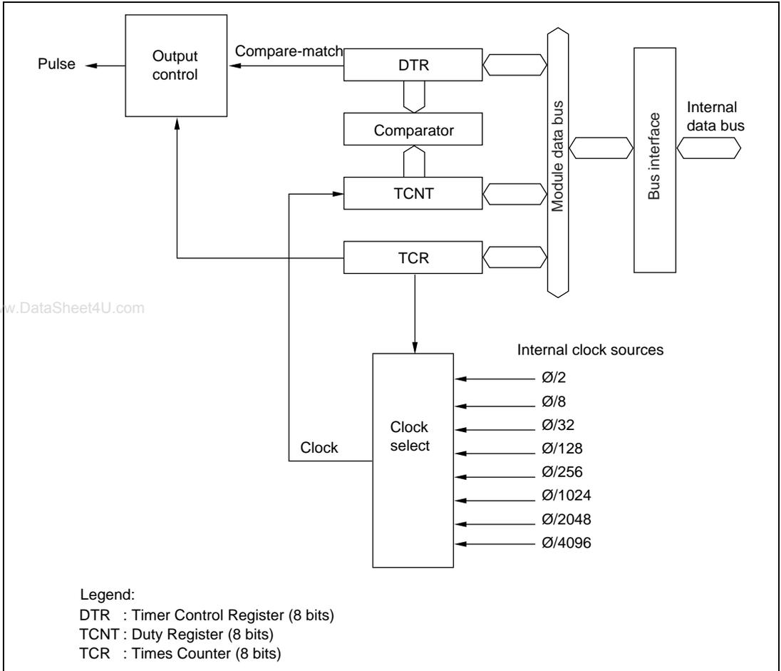
**Figure 9.1 Block Diagram of PWM Timer**
