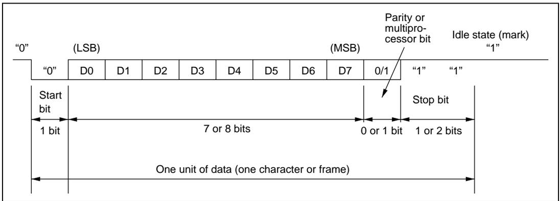
**Figure 10.2 Data Format in Asynchronous Mode**
