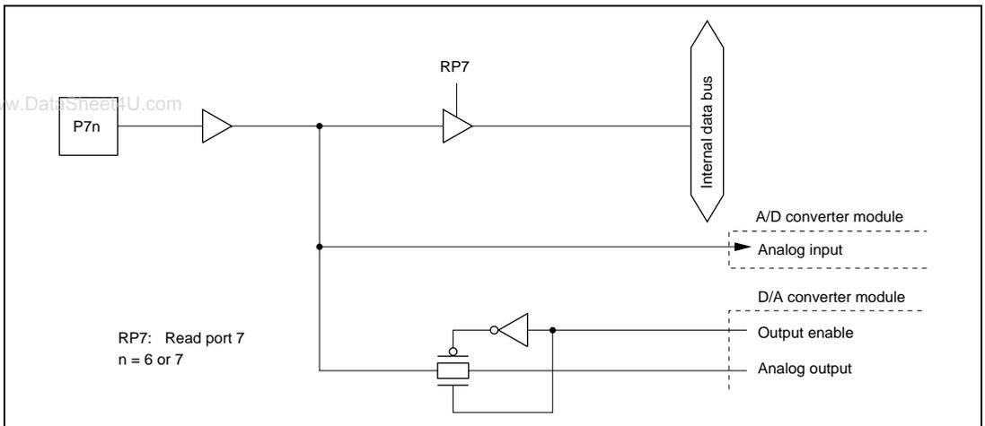
**Figure 6.7 (b) Port 7 Schematic Diagram (Pins P7<sub>6</sub> and P7<sub>7</sub>)**
