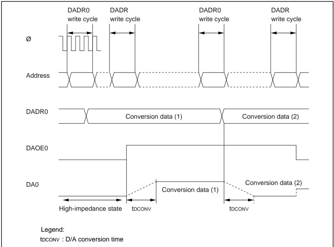
Figure 12.2 D/A Conversion (Example) [www.DataSheet4U.com](http://www.DataSheet4U.com)
