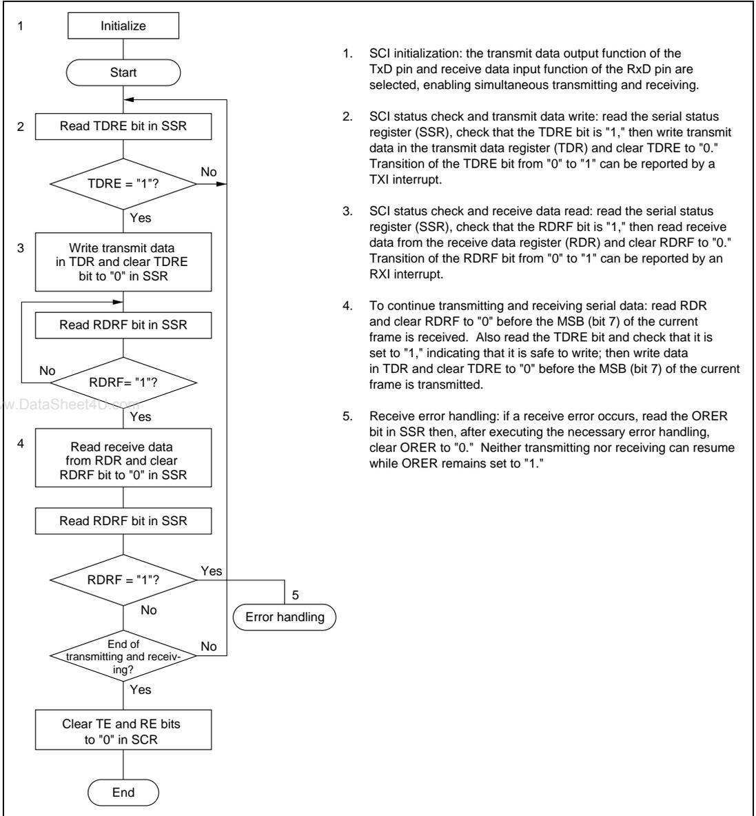
1. SCI initialization: the transmit data output function of the TxD pin and receive data input function of the RxD pin are selected, enabling simultaneous transmitting and receiving.
