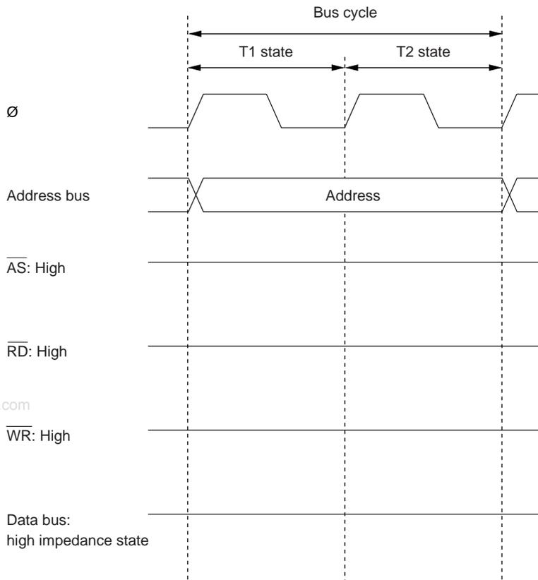
**Figure 2.14 Pin States during On-Chip Memory Access Cycle**
