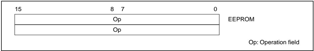
**Figure 2.10 Block Data Transfer Instruction/EEPROM Write Operation Code**
