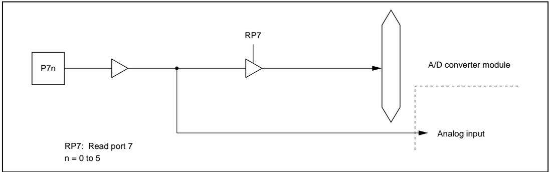
**Figure 6.7 (a) Port 7 Schematic Diagram (Pins P7<sub>0</sub> to P7<sub>5</sub>)**
