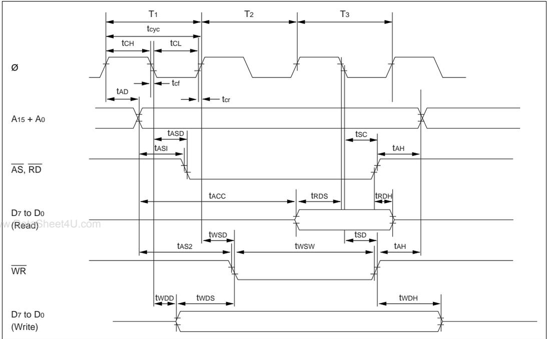
Figure 16.4 Basic Bus Cycle (without wait states) in Expanded Modes
