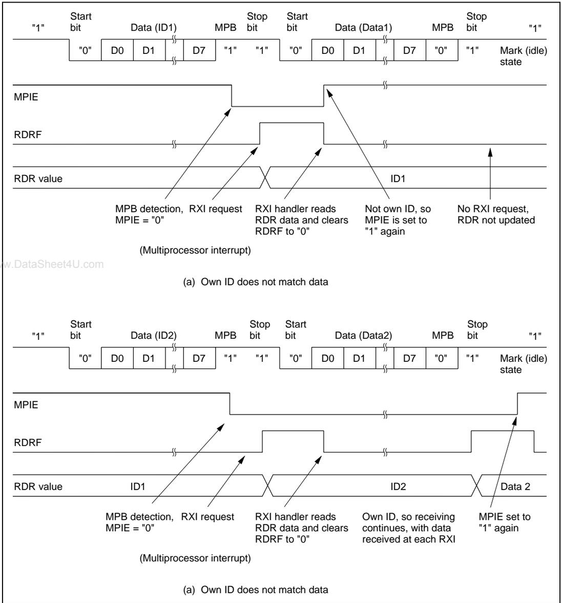
**Figure 10.11 Example of SCI Receive Operation
