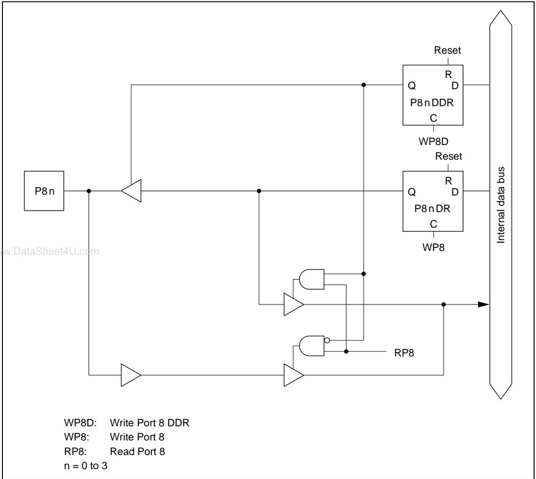
**Figure 6.8 (a) Port 8 Schematic Diagram (Pins P8<sub>0</sub> to P8<sub>3</sub>)**
