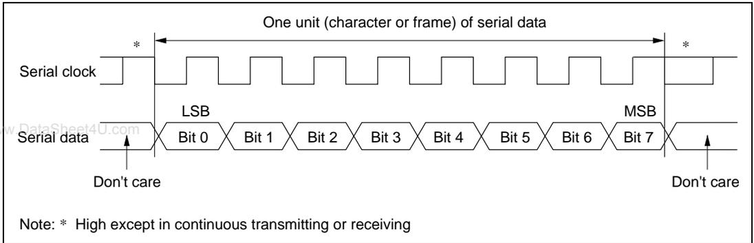
**Figure 10.12 Data Format in Clocked Synchronous Communication**
