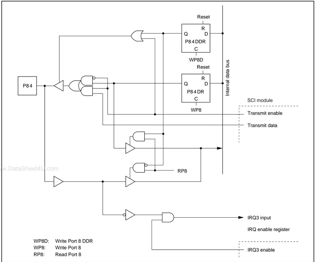
Figure 6.8 (b) Port 8 Schematic Diagram (Pin P8<sub>4</sub>)
