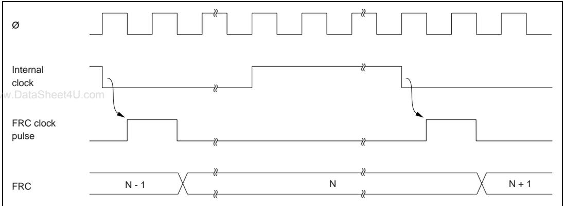
**Figure 7.4 Increment Timing for Internal Clock Source**
