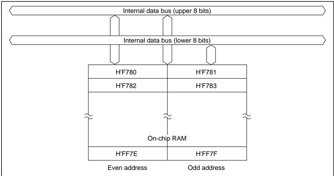
**Figure 13.1 Block Diagram of On-Chip RAM (H8/338)**
