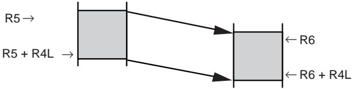
2. When setting R4L and R6, make sure that the final destination address (R6 + R4L) does not exceed H'FFFF. The value in R6 must not change from H'FFFF to H'0000 during execution of the instruction.
