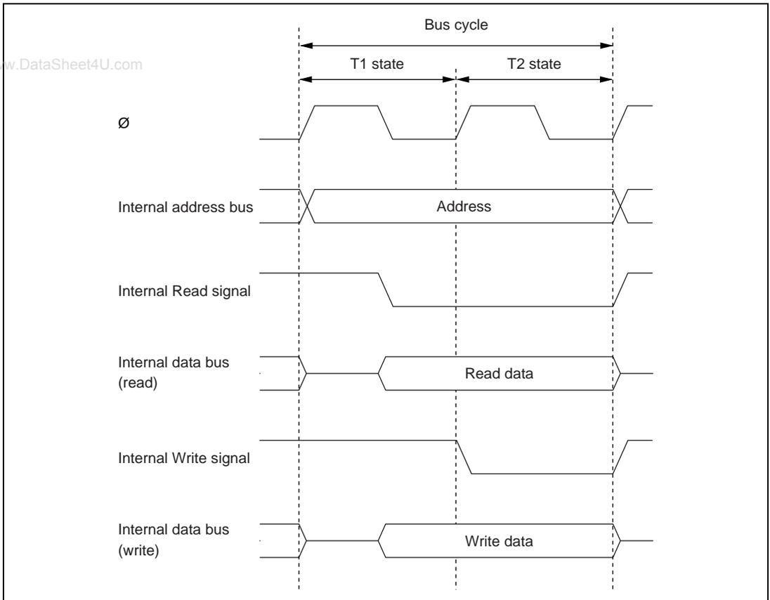
Figure 2.13 On-Chip Memory Access Cycle
