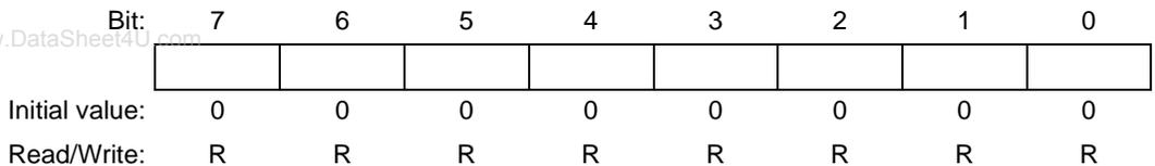
The RDR stores received data. As each character is received, it is transferred from the RSR to the RDR, enabling the RSR to receive the next character. This double-buffering allows the SCI to receive data continuously.
