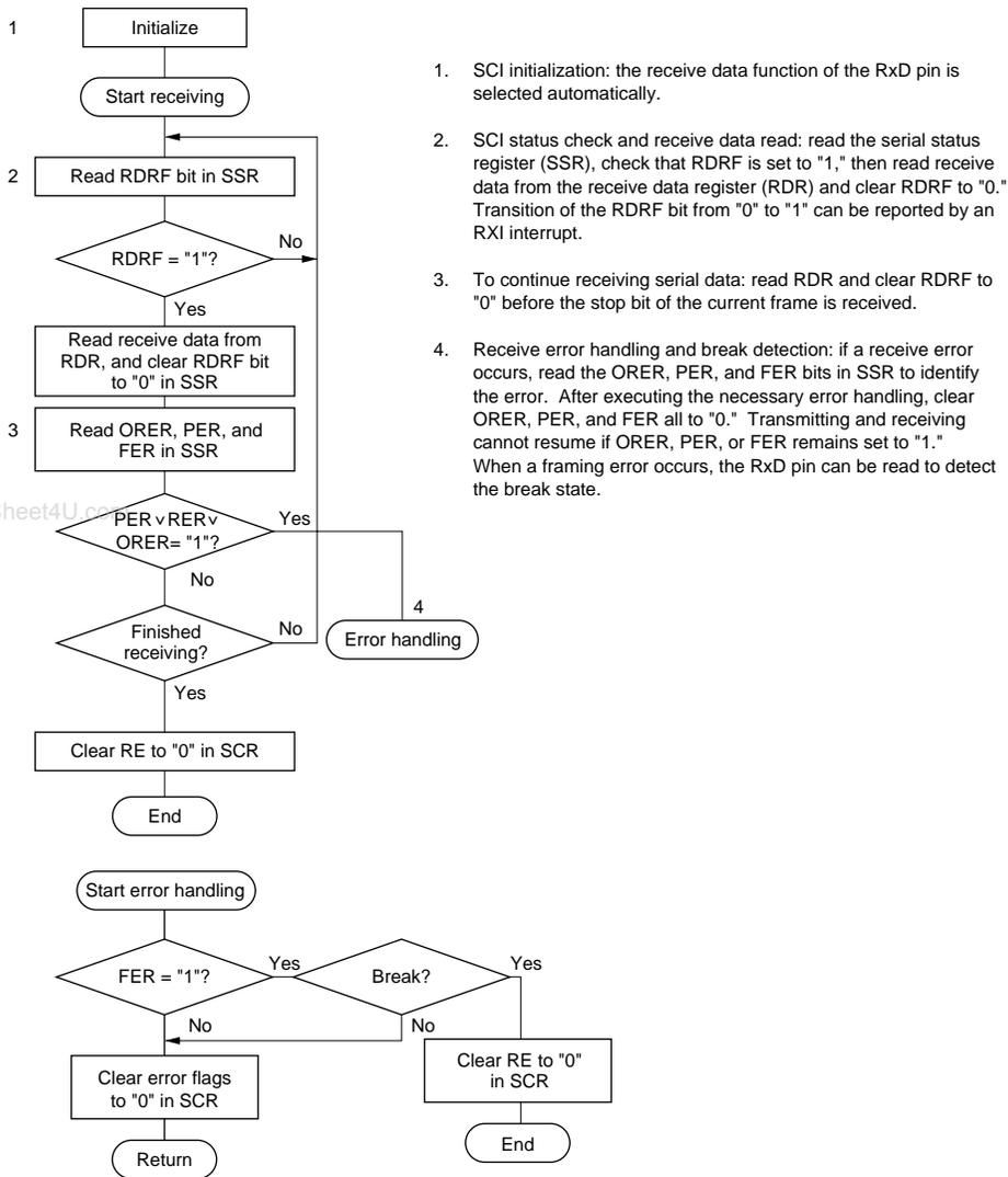
**Figure 10.7 Sample Flowchart for Receiving Serial Data**
