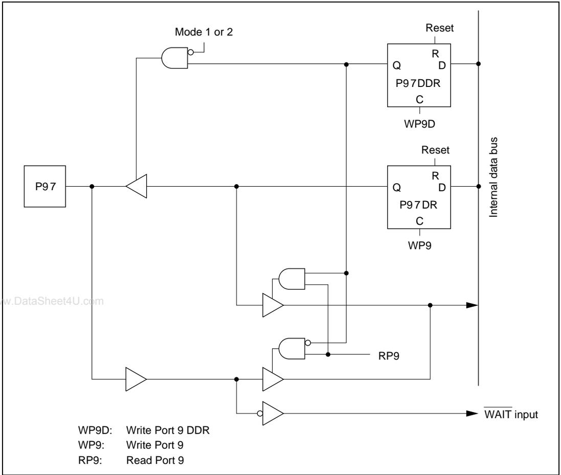
**Figure 6.9 (e) Port 9 Schematic Diagram (Pin P9<sub>1</sub>)**
