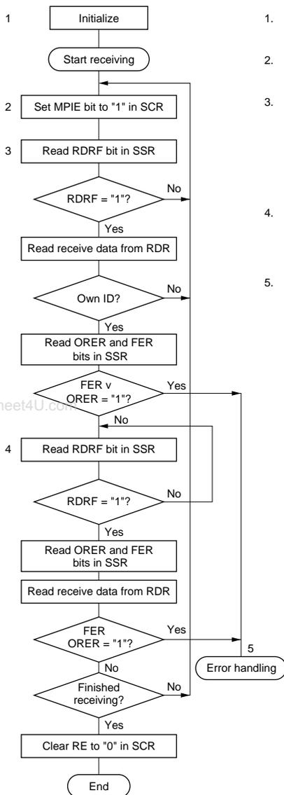
1. SCI initialization: the receive data function of the RxDPin is selected automatically.
