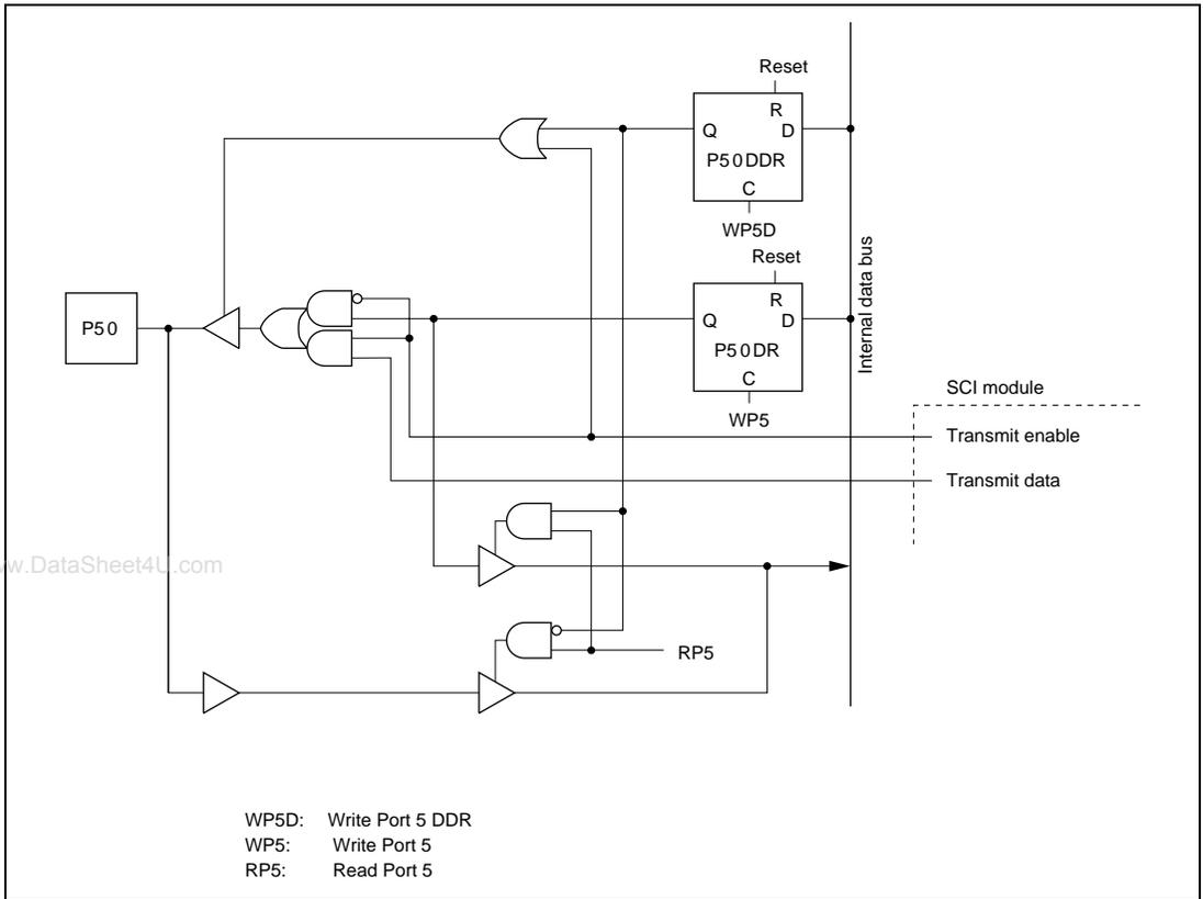
Figure 6.5 (a) Port 5 Schematic Diagram (Pin P5<sub>0</sub>)
