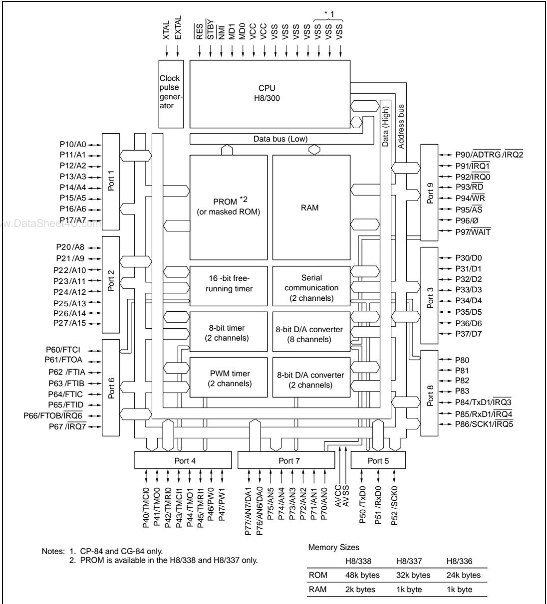
Figure 1.1 Block Diagram
