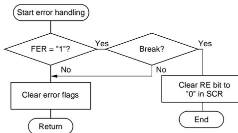
**Figure 10.10 Sample Flowchart for Receiving Multiprocessor Serial Data**
