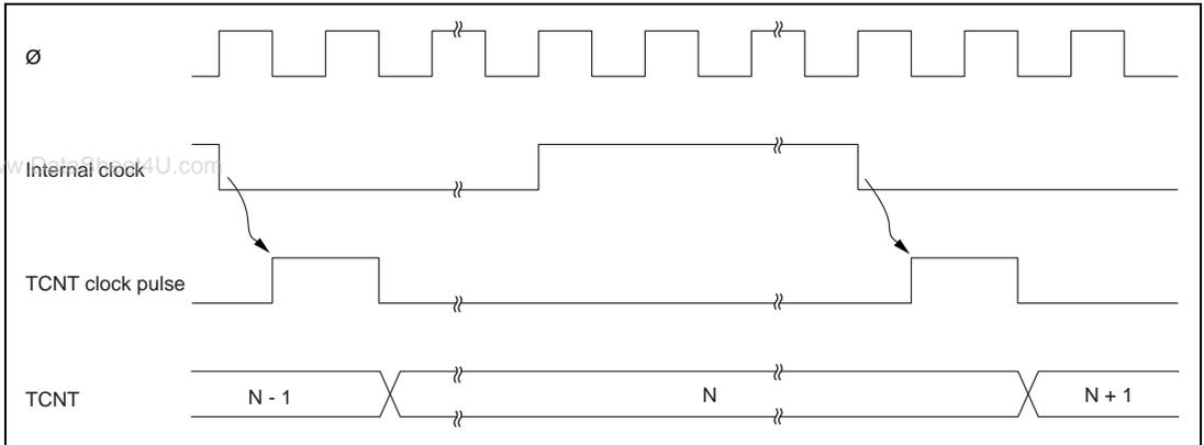
**Figure 8.2 Count Timing for Internal Clock Input**
