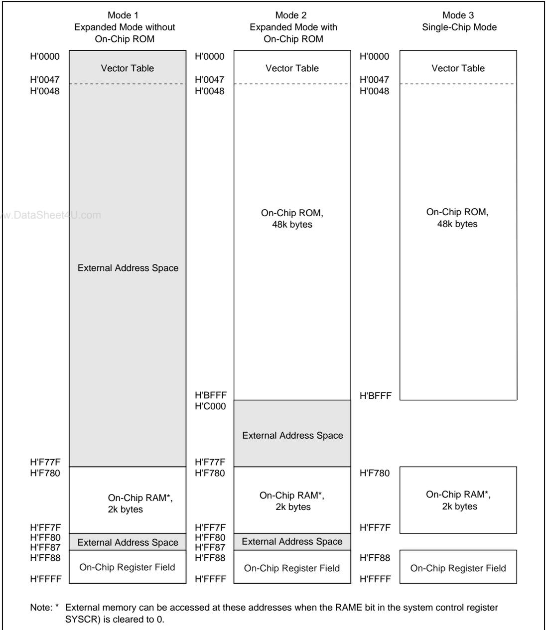
Figure 3.1 H8/338 Address Space Map [www.DataSheet4U.com](http://www.DataSheet4U.com)
