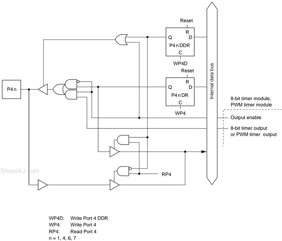
**Figure 6.4 (b) Port 4 Schematic Diagram (Pins P4<sub>1</sub>, P4<sub>4</sub>, P4<sub>6</sub>, and P4<sub>7</sub>)**
