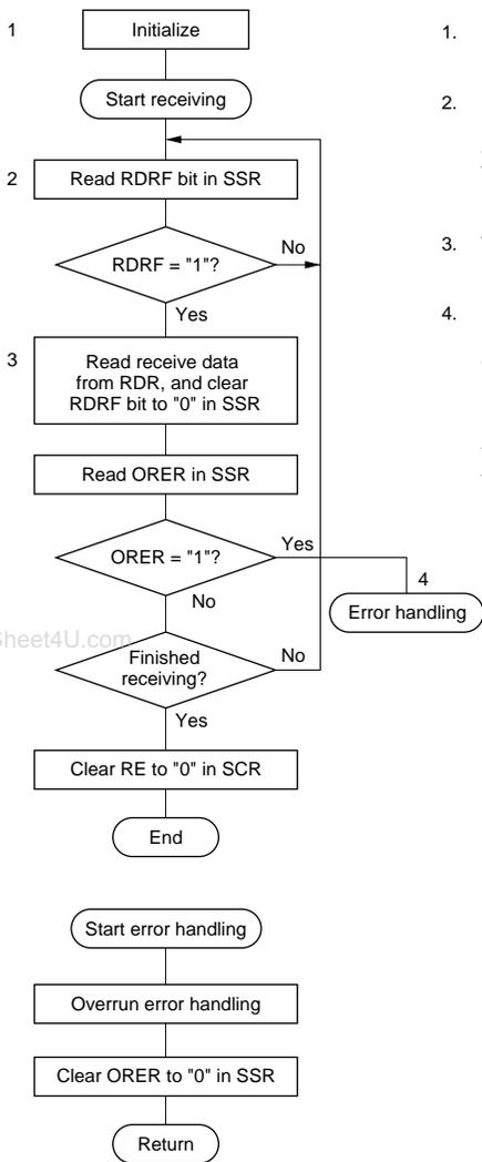
1. SCI initialization: the receive data function of the RxD pin is selected automatically.
