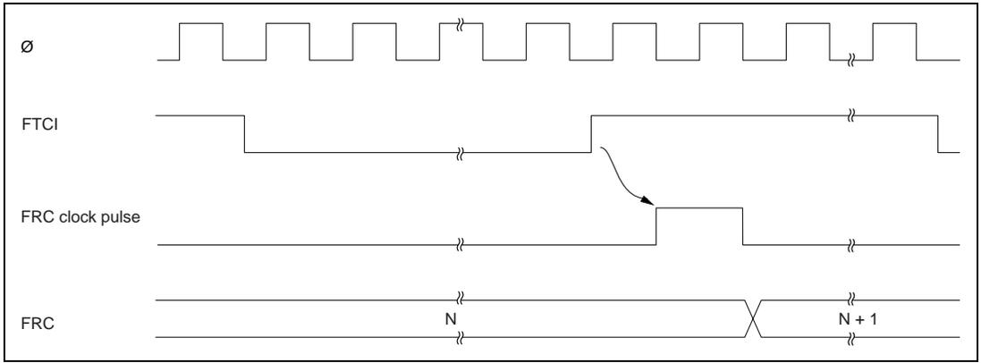
**Figure 7.5 Increment Timing for External Clock Source**
