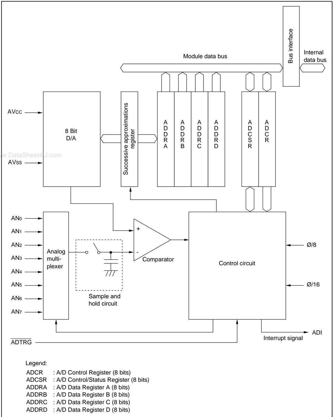
Figure 11.1 Block Diagram of A/D Converter [www.DataSheet4U.com](http://www.DataSheet4U.com)
