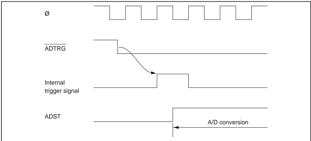
**Figure 11.5 External Trigger Input Timing**
