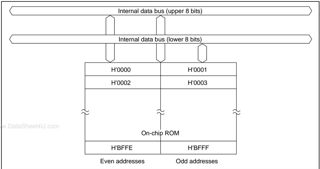
**Figure 14.1 Block Diagram of On-Chip ROM (H8/338)**
