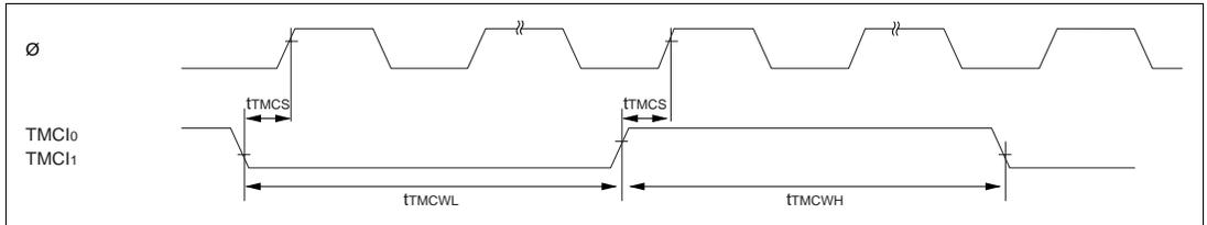
Figure 16.13 8-Bit Timer Clock Input Timing
