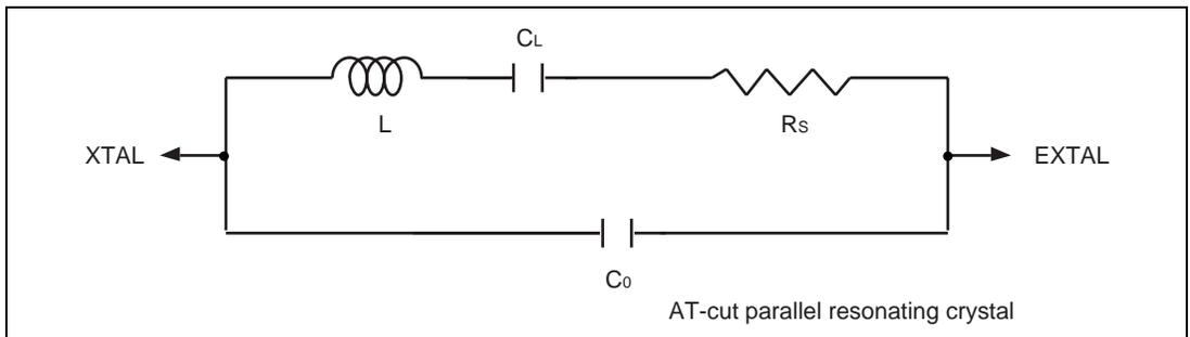
Figure 5.3 Equivalent Circuit of External Crystal
