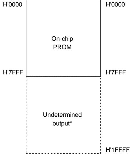
Note: \* If this address area is read in PROM mode, the output data are undetermined.
