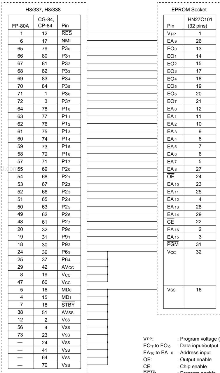
Note: All pins not listed in this figure should be left open.
