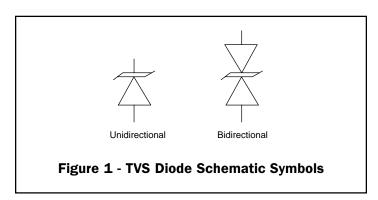
TVS diodes are available in a wide range of operating voltages. Traditional device voltages range from 5V to 440V for discrete devices. Recent innovations in TVS technology have yielded devices, such as Semtech's SLV series, which operate at 2.8 and 3.3V.
