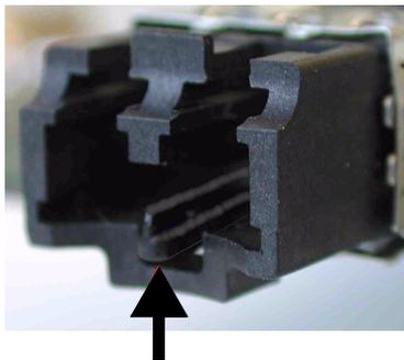
Lift here to release the transceiver from the cage
