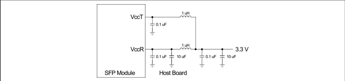
**Example SFP Host Board Schematic**
