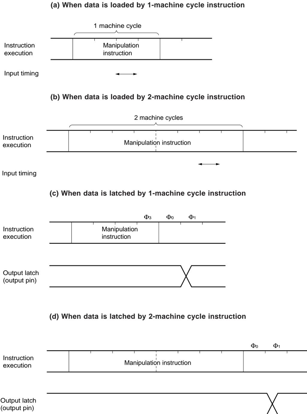
**Fig. 5-10 ON Timing of Pull-up Resistor Connected via Software**
