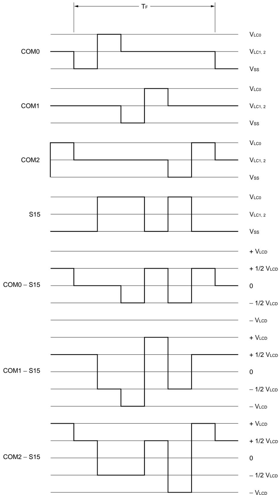
Fig. 5-121 Example of 3-Time Division LCD Drive Waveform (1/3 bias)
