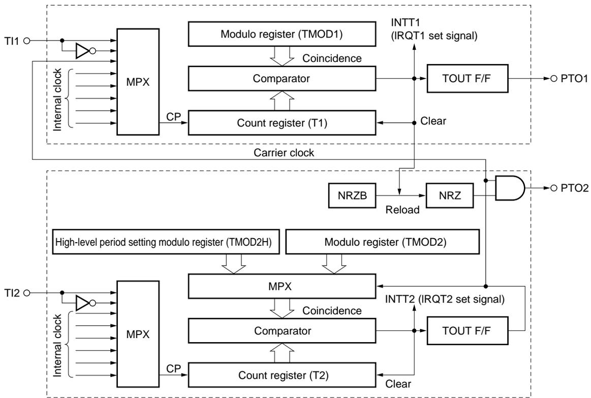
Fig. 5-57 Timing in Carrier Generator Mode
