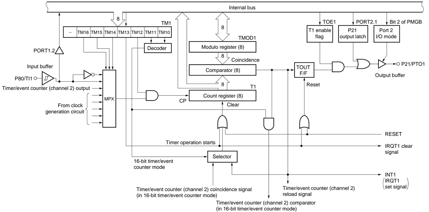
Fig. 5-30 Block Diagram of Timer/Event Counter (Channel 2)
