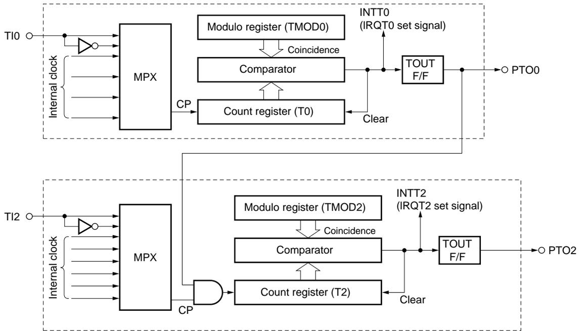
Fig. 5-42 Timing of Event Counter Operation
