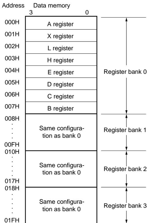
Fig. 4-7 Configuration of Register Pair
