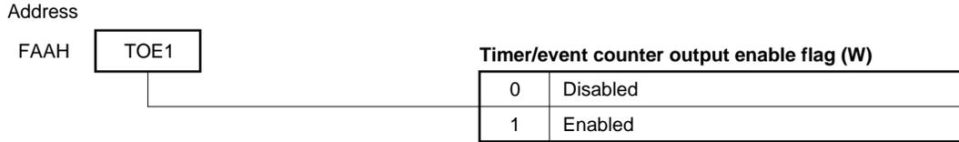
**Fig. 5-55 Setting of Timer/Event Counter Control Register**
