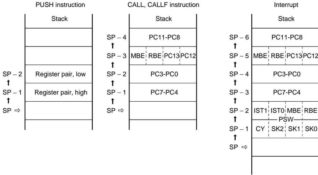
Fig. 4-11 Data Restored from Stack Memory (Mkl Mode)
