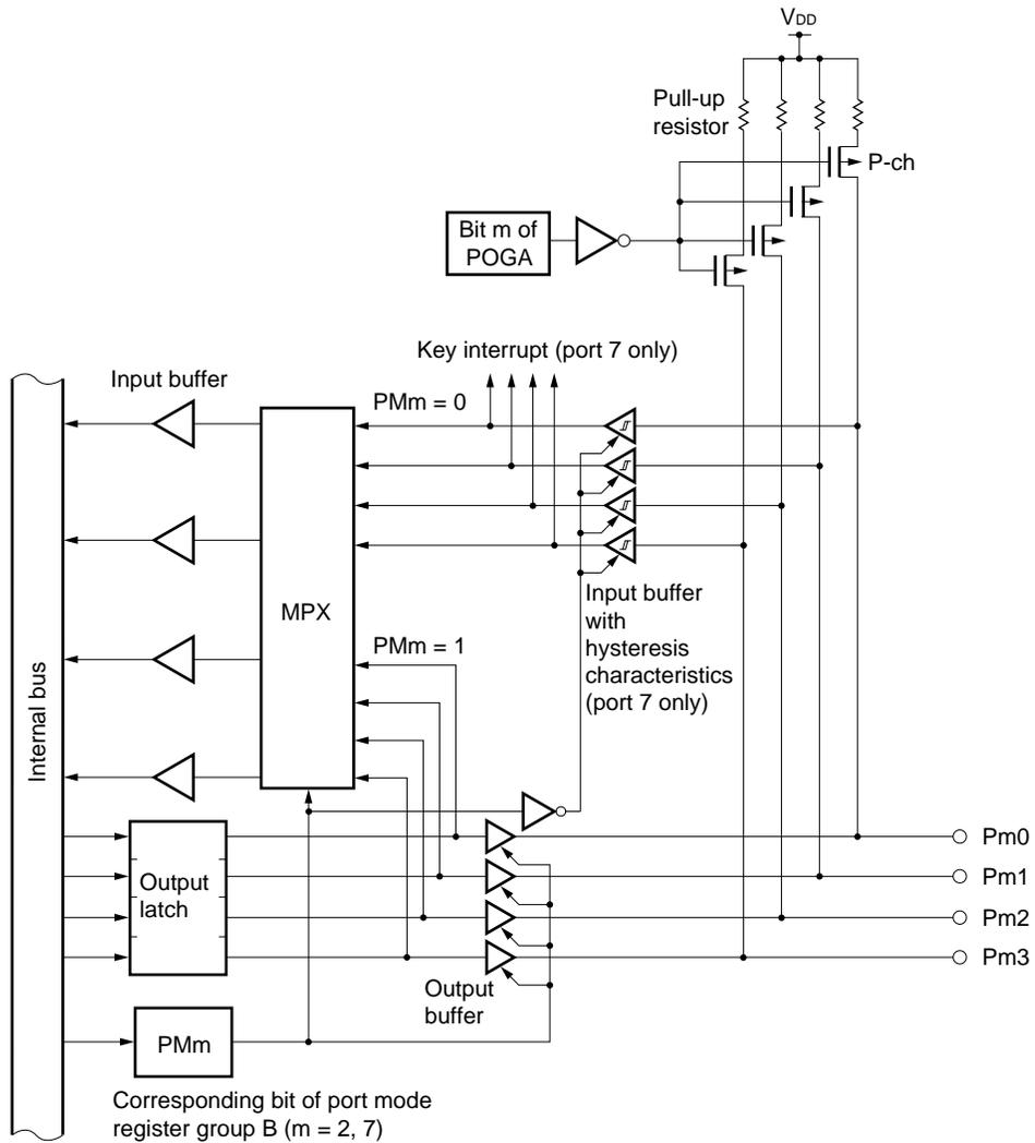
Fig. 5-6 Configuration of Port 8
