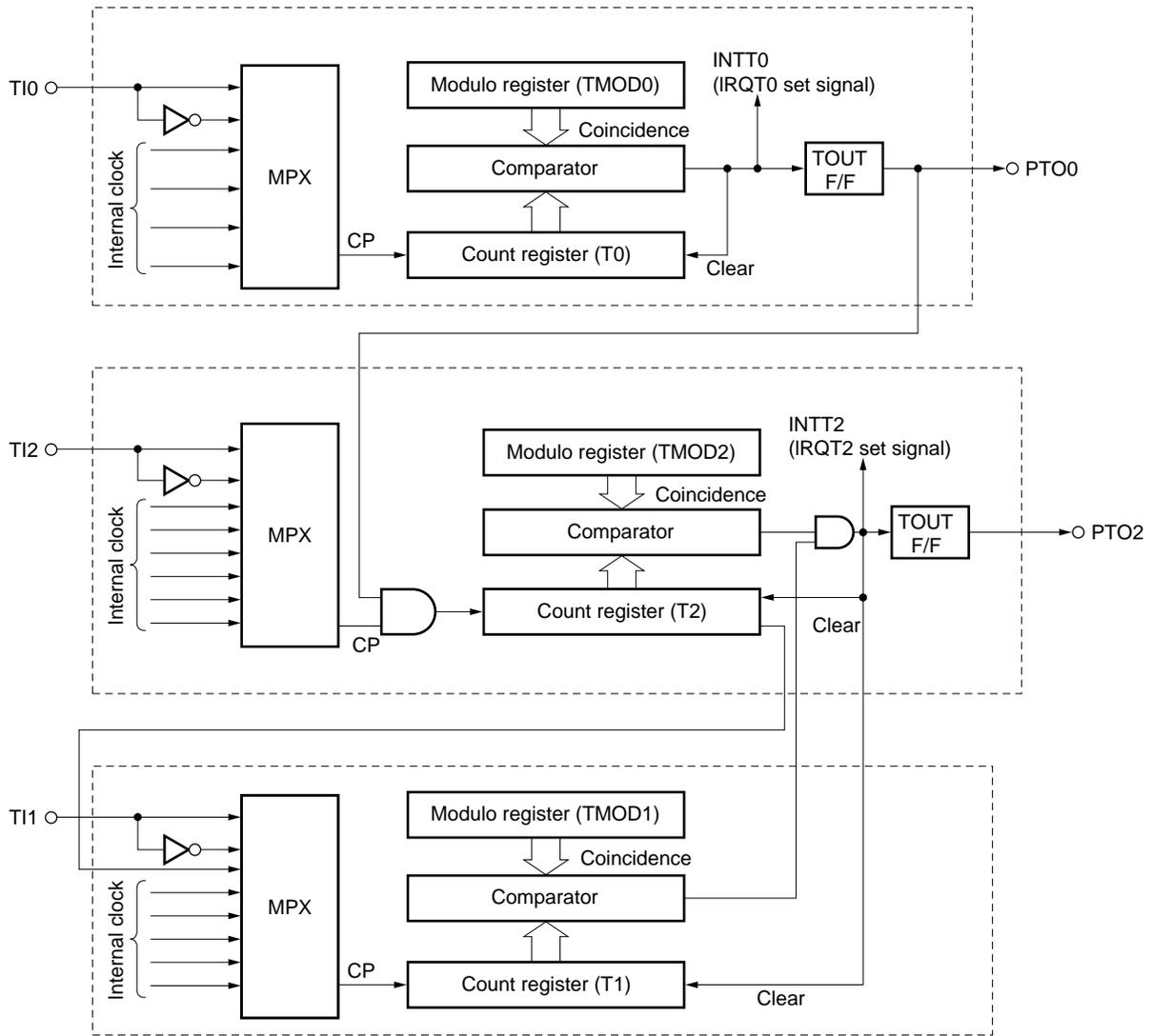
Fig. 5-52 Timing of Event Counter Operation
