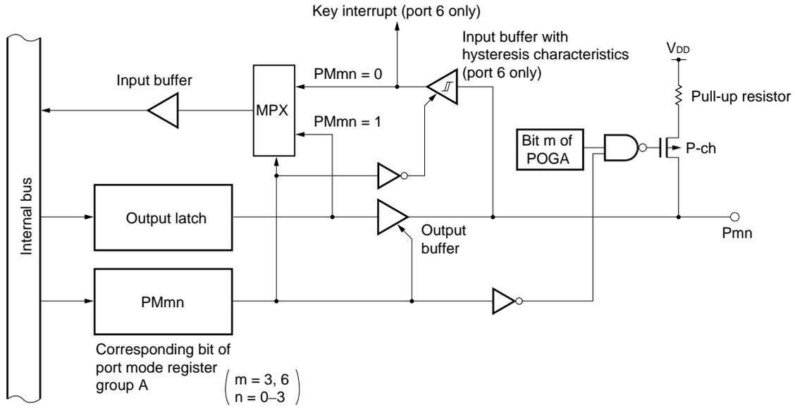
Fig. 5-4 Configuration of Ports 2 and 7
