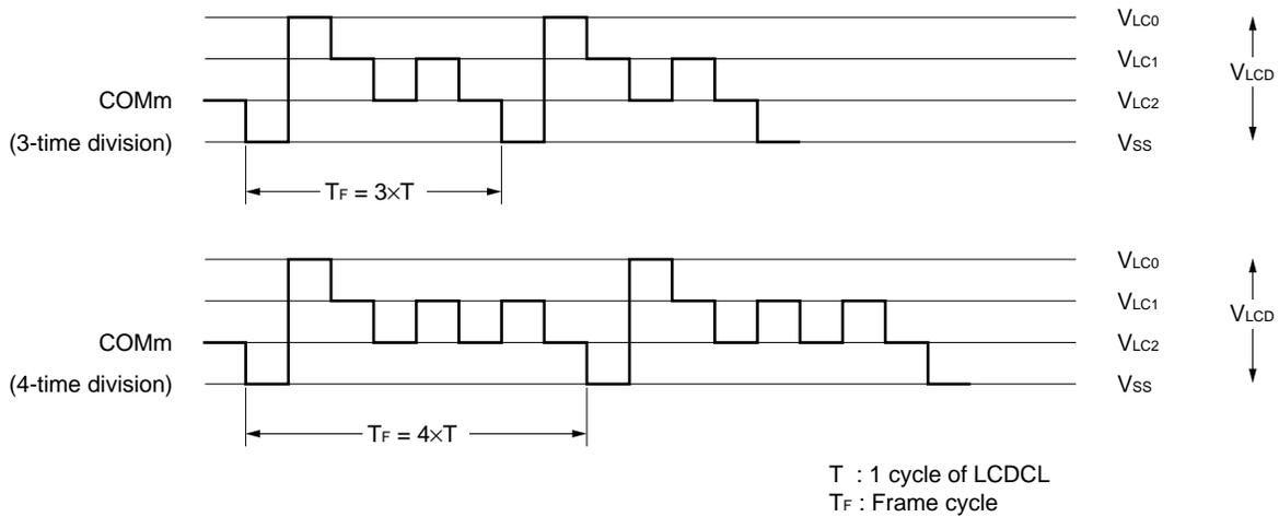
Fig. 5-109 Voltages and Phases of Common and Segment Signals
