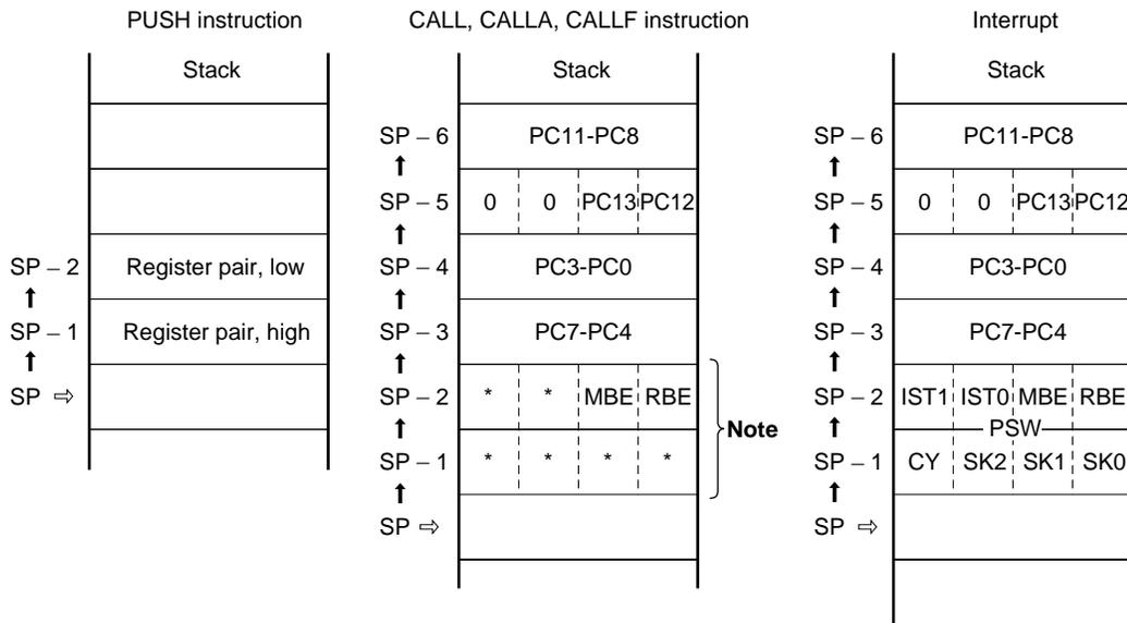
Fig. 4-13 Data Restored from Stack Memory (MkII Mode)
