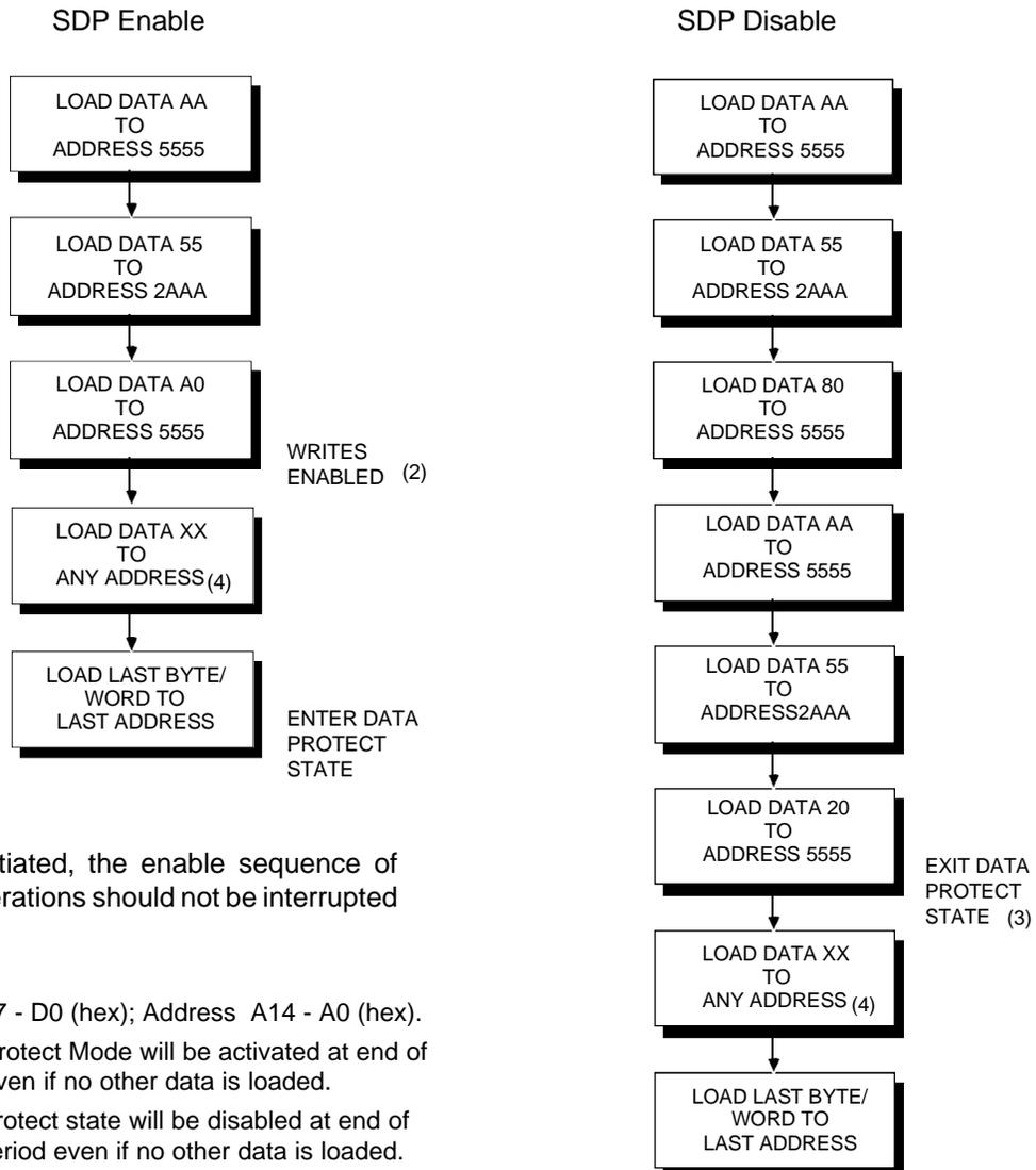
Once initiated, the enable sequence of write operations should not be interrupted
