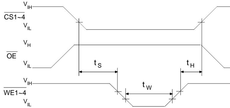
$$t_s = t_h = 5\mu\text{s (min)} \quad t_w = 10 \text{ ms (min)} \quad V_H = 12\text{V} \pm 0.5\text{V}$$
