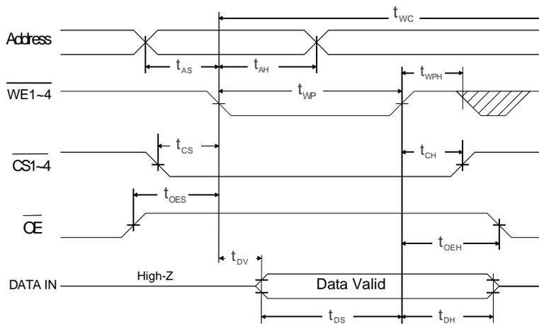
**AC Write Waveform - CS1~4 Controlled**
