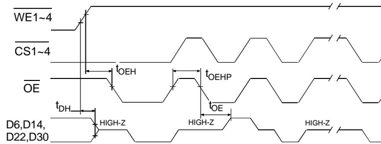
**Software Protected Write Waveform (1,2)**
