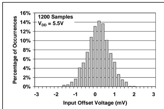
**FIGURE 2-4:** Input Offset Voltage at  $V_{DD} = 5.5\text{V}$ .
