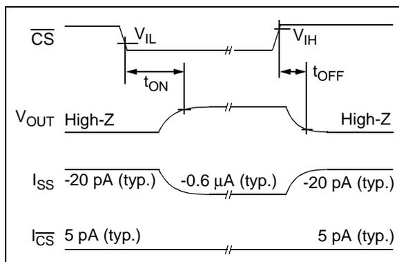
**FIGURE 1-1:** Chip Select ( $\overline{CS}$ ) Timing Diagram (MCP6143 only).
