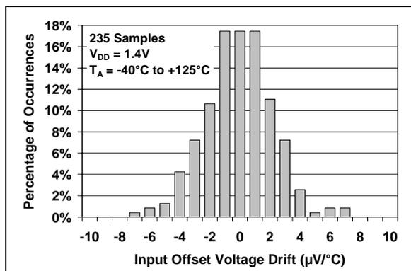
**FIGURE 2-2:** Input Offset Voltage Drift at  $V_{DD} = 1.4\text{V}$ .
