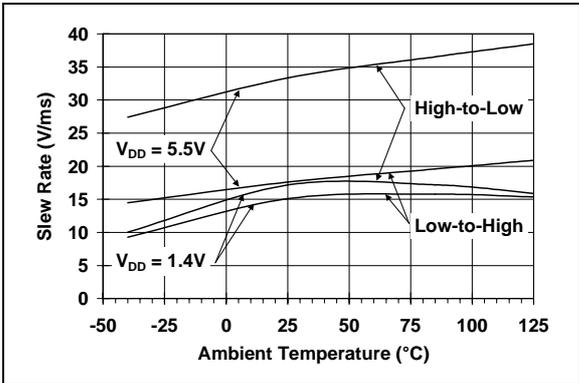
**FIGURE 2-26:** Slew Rate vs. Ambient Temperature.
