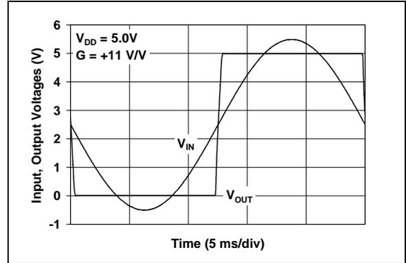
**FIGURE 2-10:** The MCP6141/2/3/4 family shows no phase reversal.
