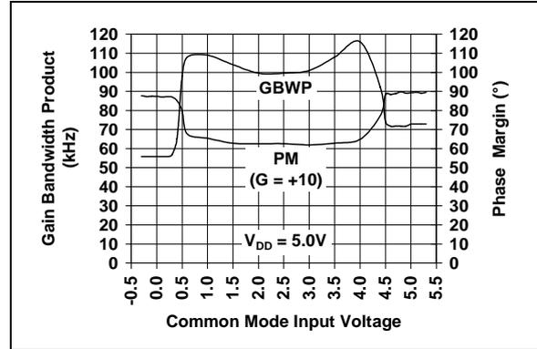
**FIGURE 2-22:** Gain Bandwidth Product, Phase Margin vs. Common Mode Input Voltage.
