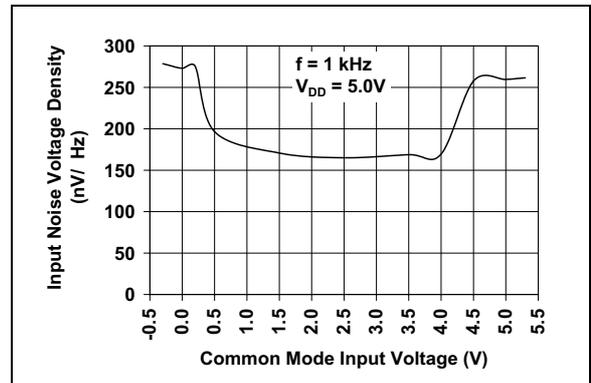
**FIGURE 2-11:** Input Noise Voltage Density vs. Common Mode Input Voltage.
