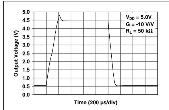
**FIGURE 2-33:** Large Signal Inverting Pulse Response.
