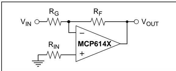
**FIGURE 4-3:** Noise Gain for Inverting Gain Configuration.
