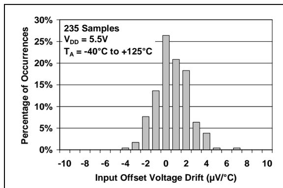
**FIGURE 2-5:** Input Offset Voltage Drift at  $V_{DD} = 5.5\text{V}$ .
