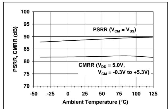
**FIGURE 2-12:** CMRR, PSRR vs. Ambient Temperature.
