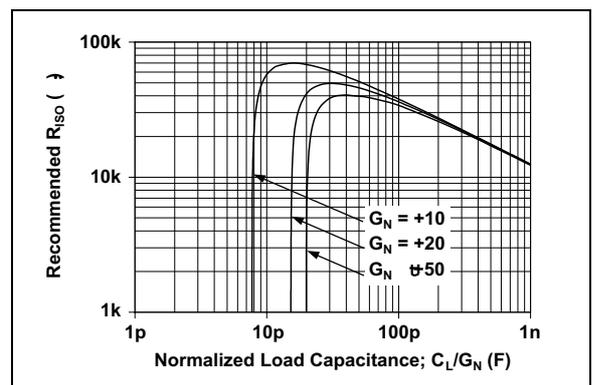
**FIGURE 4-6:** Recommended  $R_{ISO}$  Values for Capacitive Loads.
