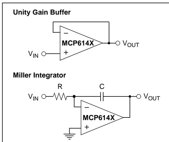
**FIGURE 4-4:** Typical Unstable Circuits for the MCP6141/2/3/4 Family.
