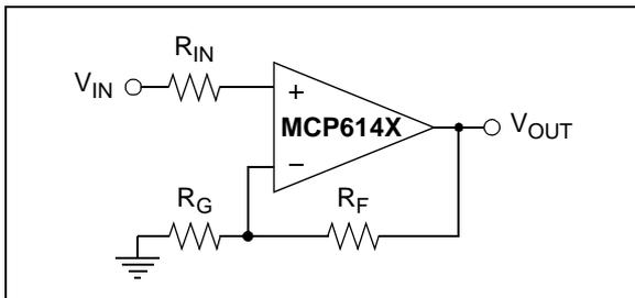
**FIGURE 4-2:** Noise Gain for Non-inverting Gain Configuration.
