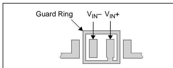
FIGURE 4-8: Example Guard Ring Layout for Inverting Gain.
