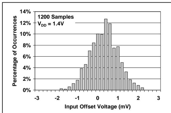
**FIGURE 2-1:** Input Offset Voltage at  $V_{DD} = 1.4\text{V}$ .
