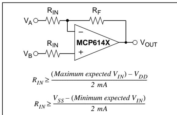
**FIGURE 4-1:** Input Current-Limiting Resistor ( $R_{IN}$ ).
