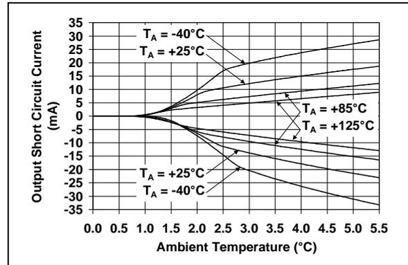
**FIGURE 2-24:** Output Short Circuit Current vs. Power Supply Voltage.
