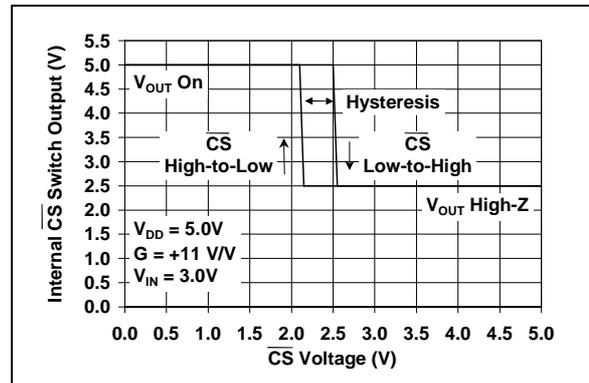
**FIGURE 2-34:** Internal Chip Select ( $\overline{\text{CS}}$ ) Hysteresis (MCP6143 only).
