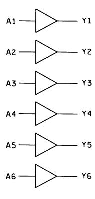
FIGURE 3. Logic diagram.
