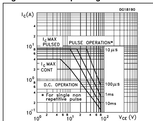
**Figure 3. Derating curve**
